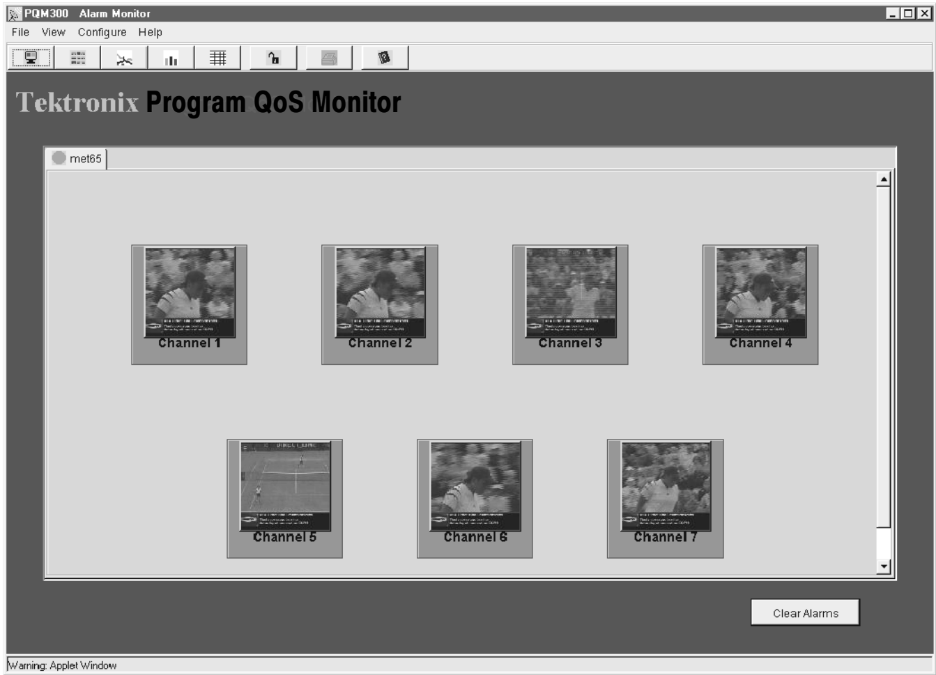
Figure 2-3: Alarm monitor by connection view
