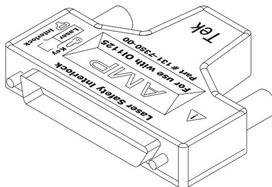
Figure 8: Laser safety interlock
