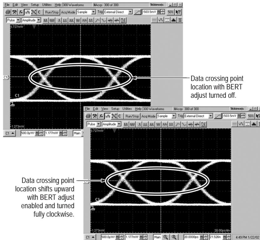
Figure 16: Using an eye pattern to check modulator polarity
