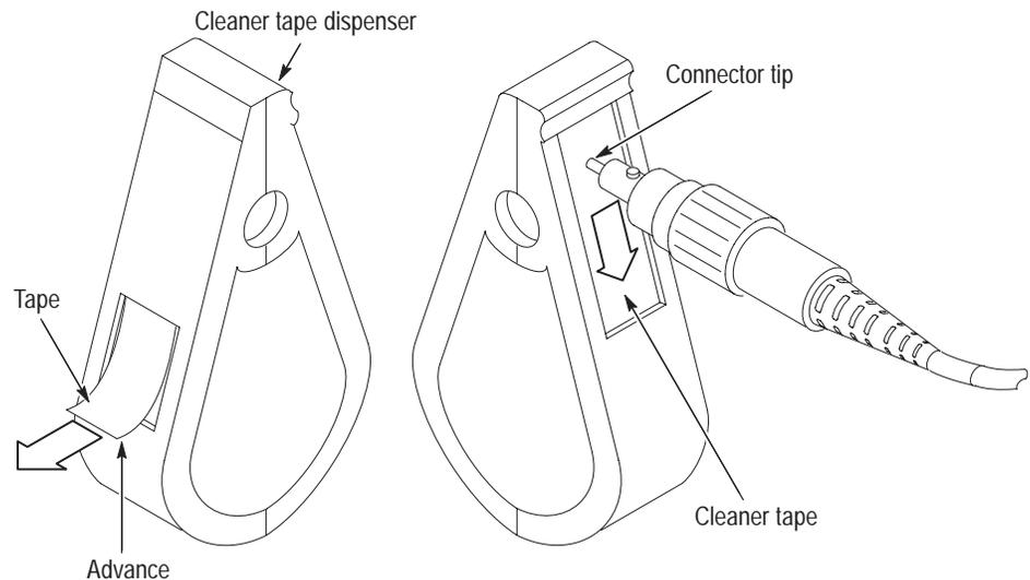
**Figure 20: Cleaning an optical connector**
