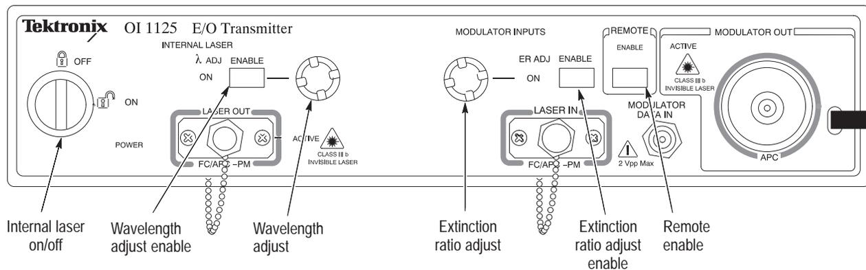
Figure 6: OI1125 front-panel controls
