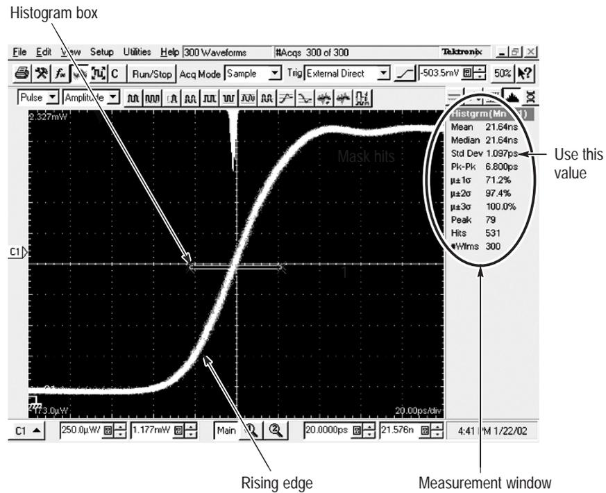
Figure 15: RMS Jitter measurement
