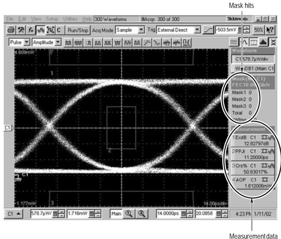
Figure 19: Measurements taken from the eye pattern
