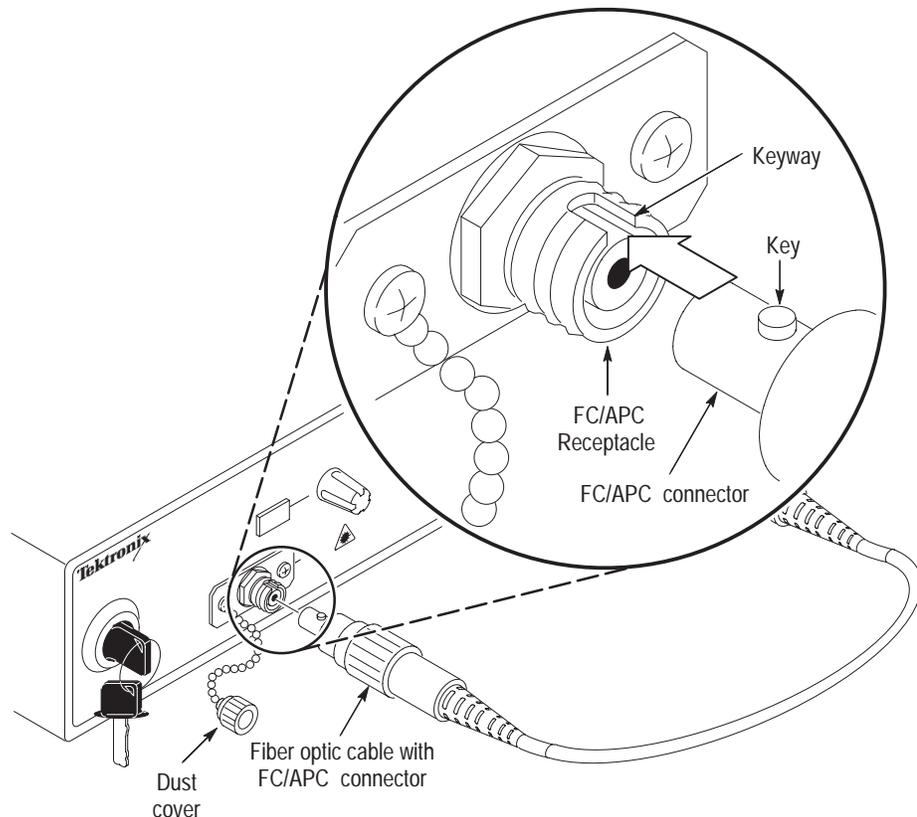
**Figure 4: Connecting a fiber optic cable**
