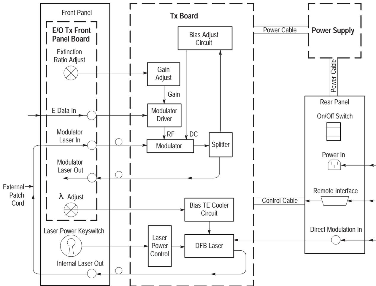
Figure 11: Transmitter interconnect diagram
