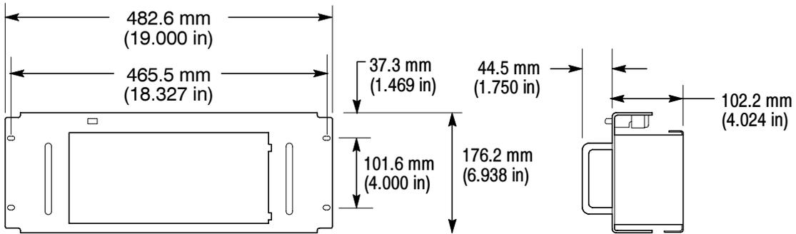
Figure 3: Dimensions of the RM2000 Rackmount
