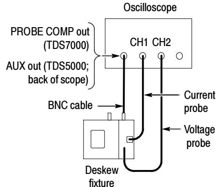
Figure 1: Typical small current probe connection
