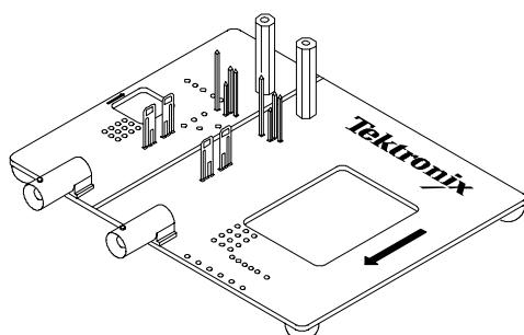
This fixture converts the PROBE COMPENSATION output of the TDS7000 or the AUX OUT output of the TDS5000 into a set of test point connections that provide you with a convenient way to compensate for timing differences between voltage and current probes.
