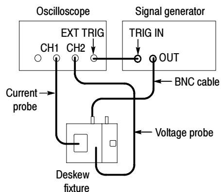
Figure 2: Typical large current probe connection using an external signal source
