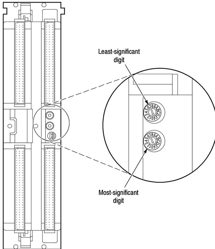
**Figure 5: Logical address switches (set to address FF)**
