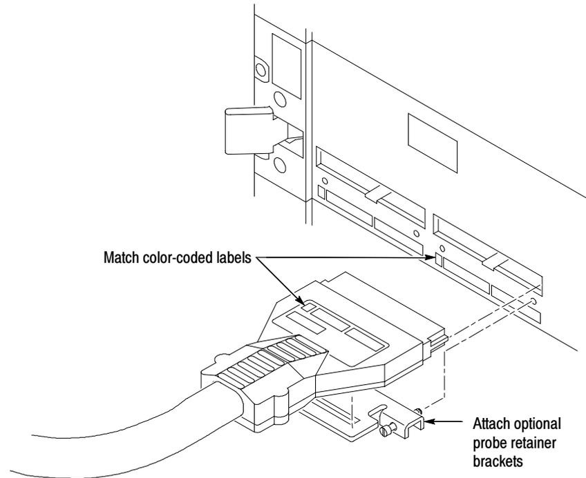
**Figure 13: Connecting the P64xx logic analyzer probes to the TLA7Lx/Mx/Nx/Px/Qx logic analyzer modules**
