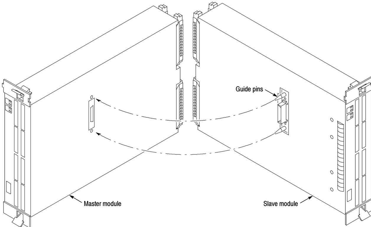
**Figure 24: Lining up the two modules**
