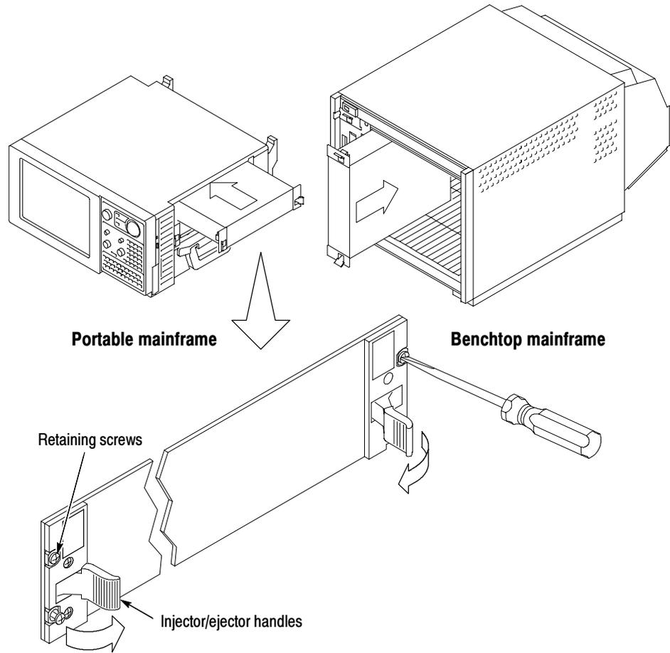
**Figure 6: Installing modules**
