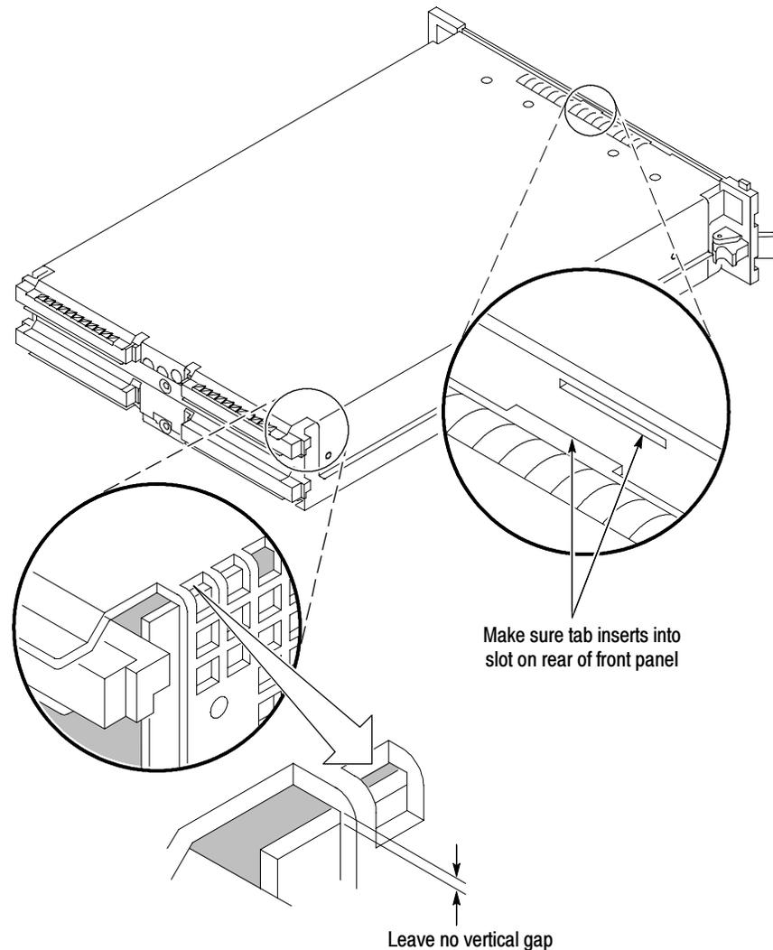
**Figure 23: Seating the cover on the chassis**
