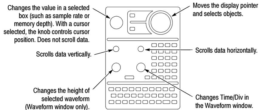
Figure 26: TLA715 Portable mainframe front panel
