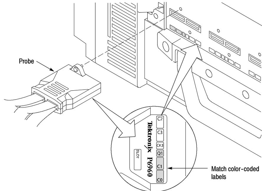
**Figure 11: Connecting the P68xx or P69xx logic analyzer probes to the TLA7NAx logic analyzer module**
