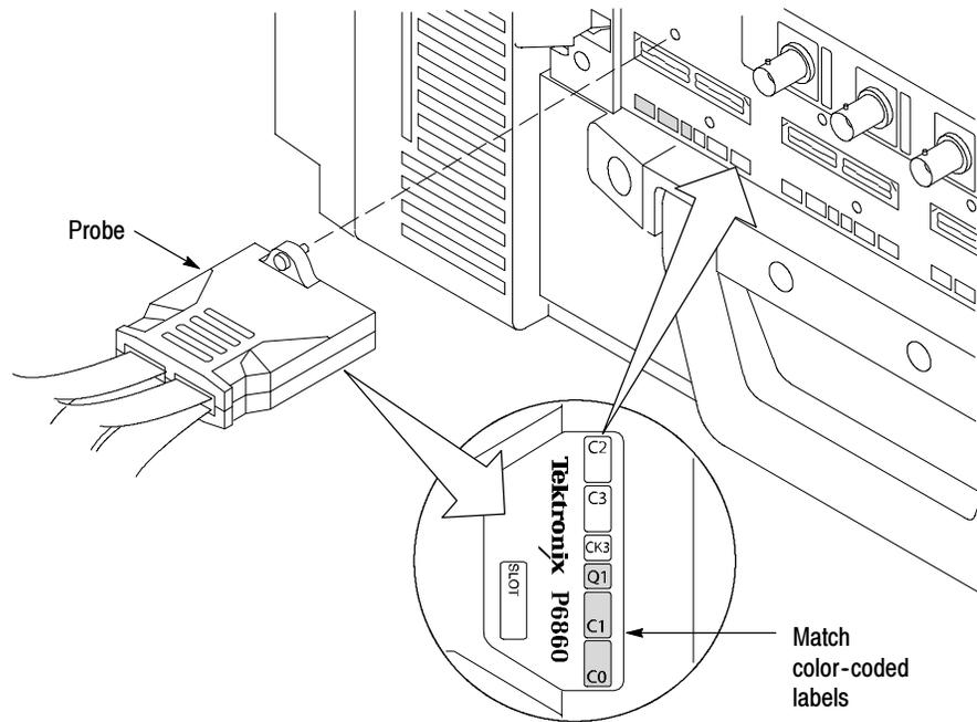
**Figure 12: Connecting the P68xx or P69xx logic analyzer probes to the TLA7Axx logic analyzer module**
