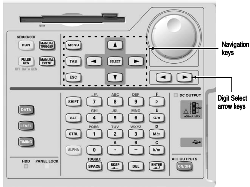
Figure 2-3: Front panel controls
