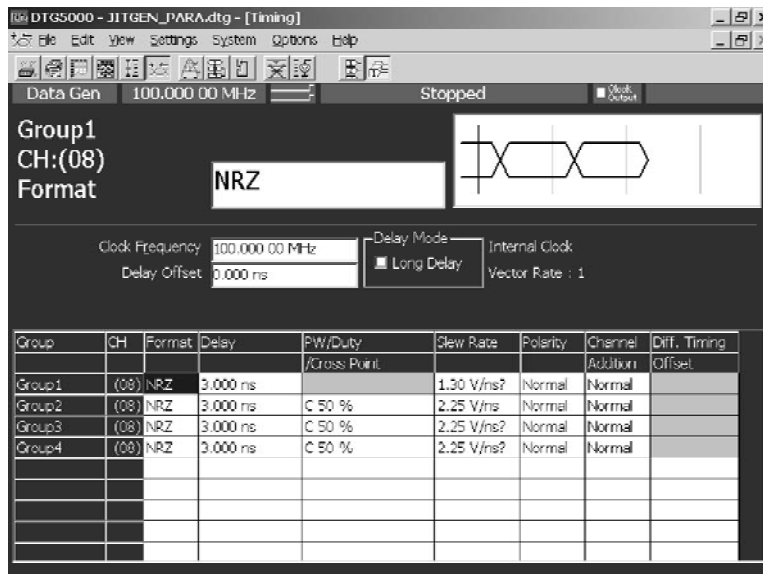
Figure 2-15: Timing window (Data Generator mode)
