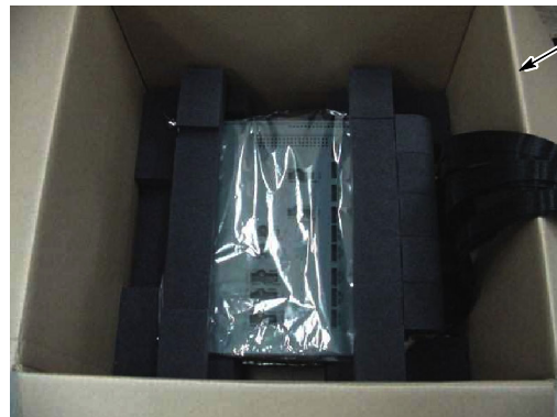
Figure 1-12: Place the preprocessor unit in the cardboard carton
