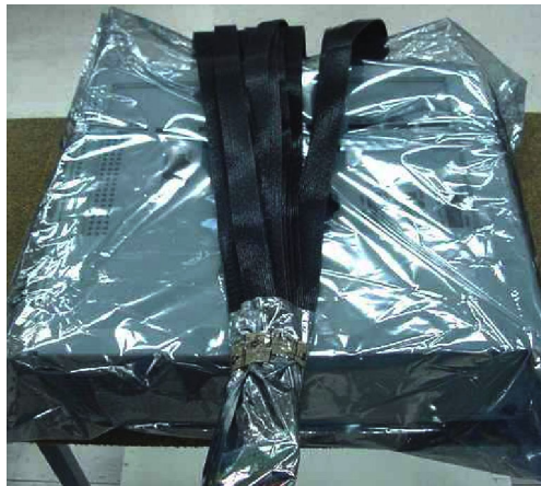
Figure 1-10: Use static-shielding bags.
