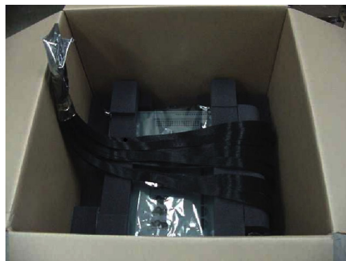
Figure 1-13: Place the cables carefully over the preprocessor unit
