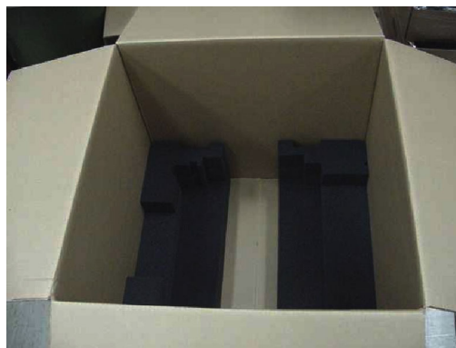
Figure 1-11: Place foam in the cardboard carton
