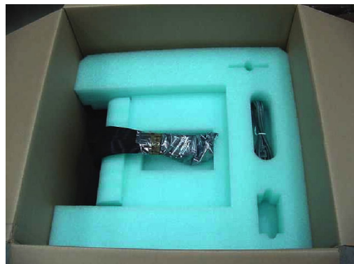
Figure 1-14: Place the foam and probe head in place
