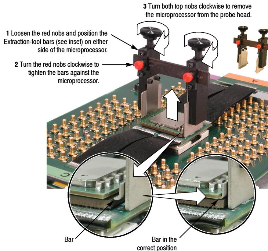
**Figure 1-7: Remove the microprocessor with the extraction tool**
