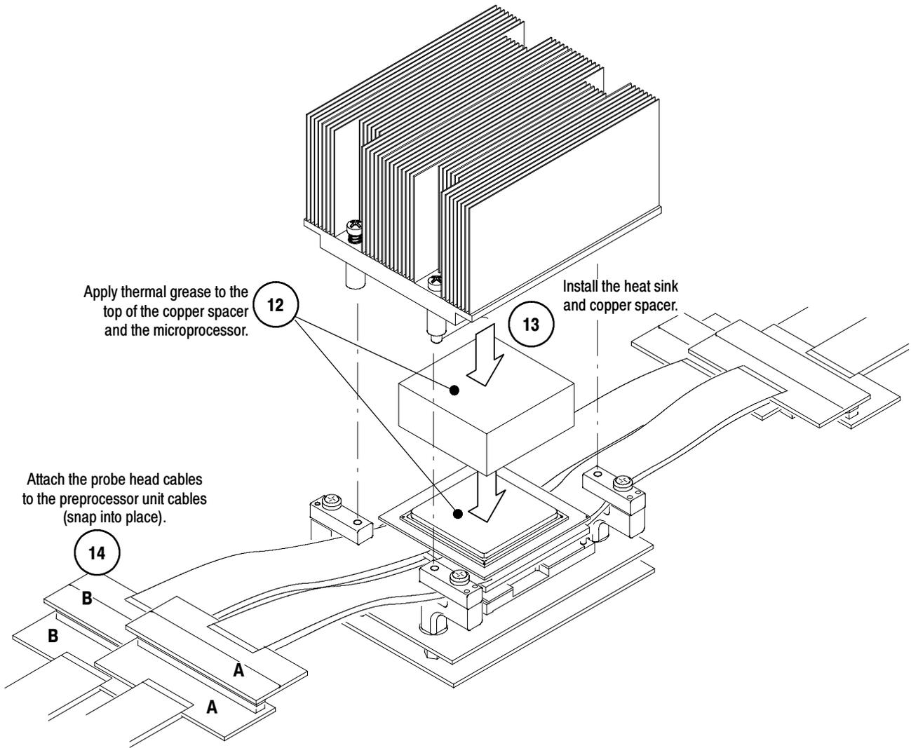
**Figure 1-6: Attaching the heat sink to the target system**
