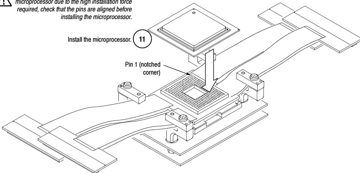
**Figure 1-5: Attaching the heat sink brackets and microprocessor to the target system**
