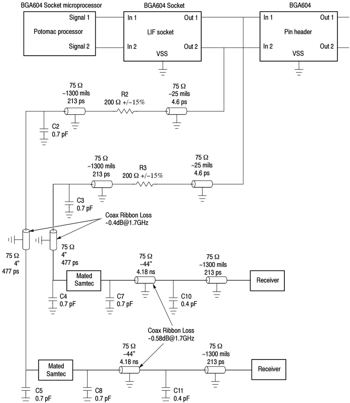
Figure 2-1: Probe adapter preliminary load model for typical signals
