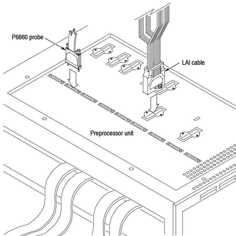
**Figure 1-9: LAI cable, P6860 probe, and preprocessor unit**
