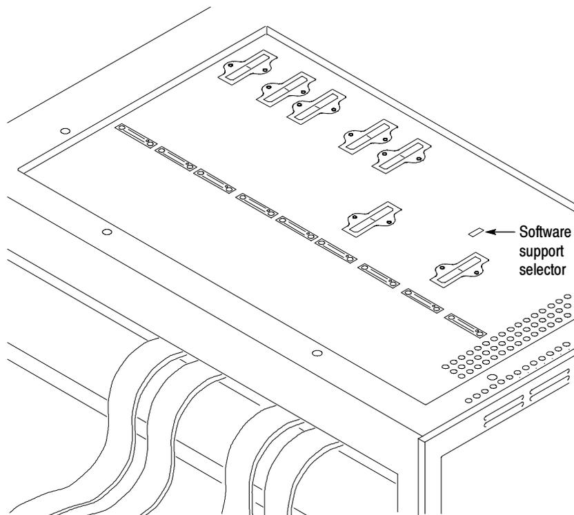
**Figure 1-2: Selecting your software on the preprocessor unit**
