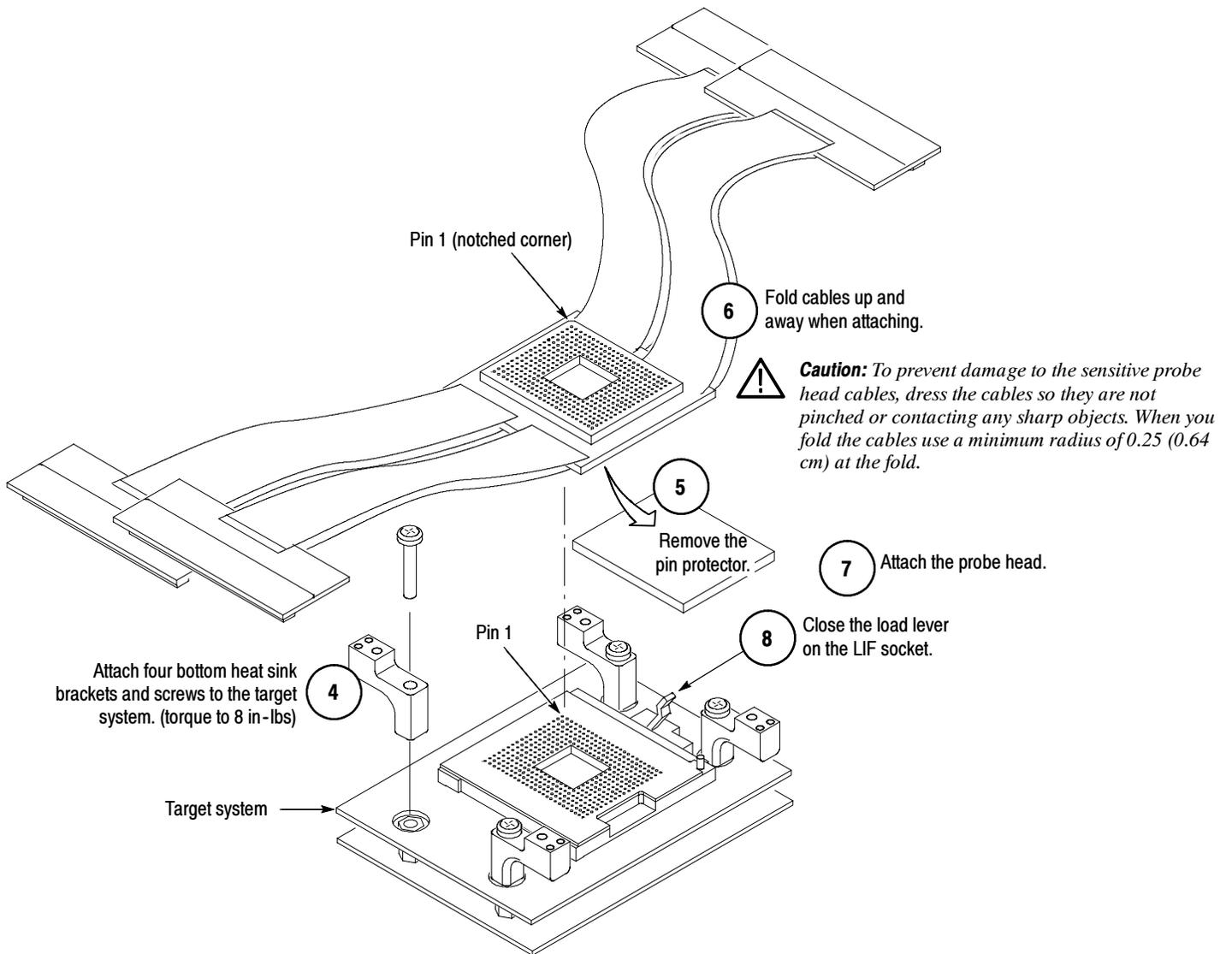
Figure 1-4: Attach the probe head to the target system
