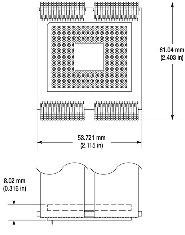
**Figure 2-6: Dimensions of the probe head**
