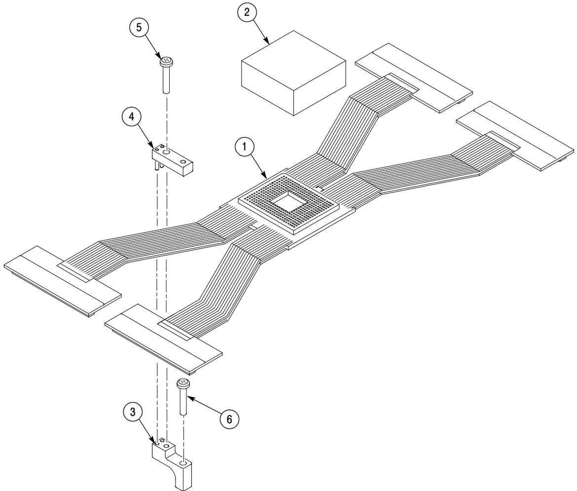
**Figure 4-1: Probe adapter exploded view**
