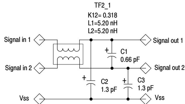
**Figure 2-3: Socket electrical load model for typical signals**
