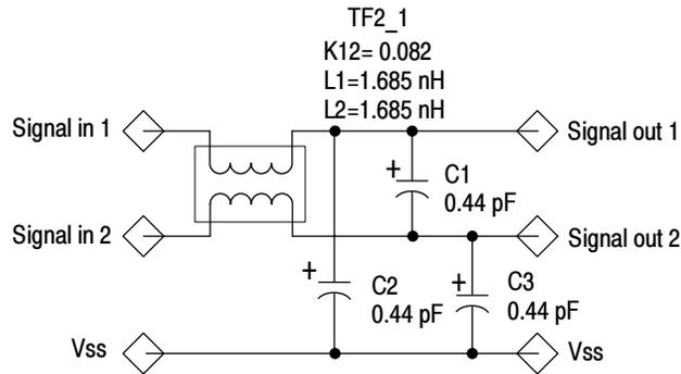
**Figure 2-2: Pin header electrical load model for typical signals**
