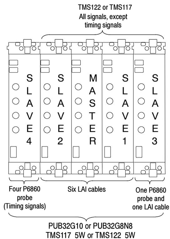
**Figure 1-10: LAI cable, P6860 probe, and module configurations**
