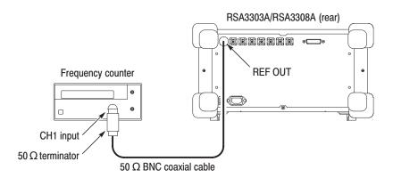
Figure 4-7: Initial test hookup
