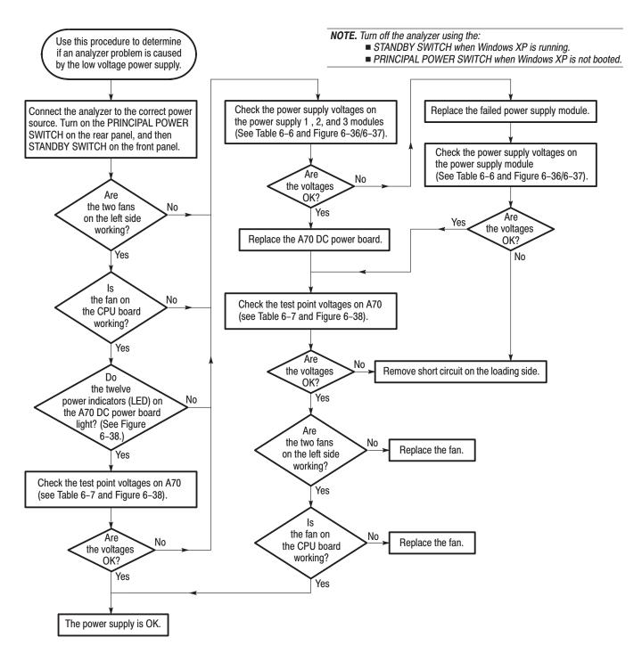
Figure 6-32: Troubleshooting procedure 1 — Power supply system
