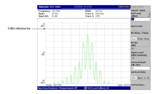
Figure 2-18: Reference level of 10 dBm
