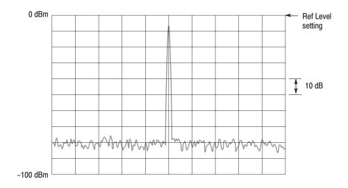
Figure 2-16: Setting amplitude
