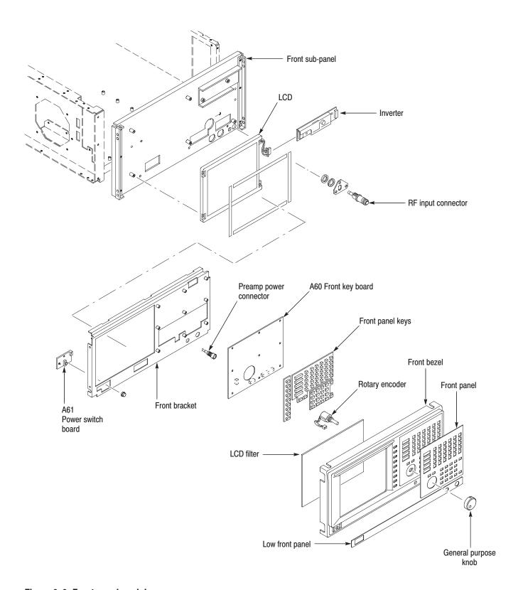
Figure 6-9: Front panel modules
