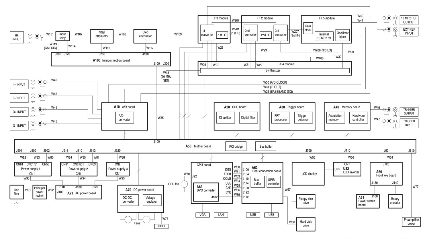
Figure 9-2: Interconnect diagram (RSA3303A)
