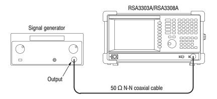
Figure 4–11: Hookup for checking the absolute amplitude accuracy
