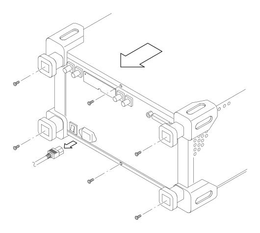
Figure 6-12: Line cord and cabinet removal
