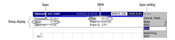
Figure 4-2: Setup display
