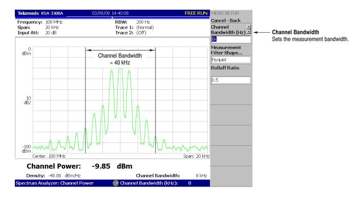
Figure 2-29: Channel power measurement (Channel Bandwidth = 40 kHz)
