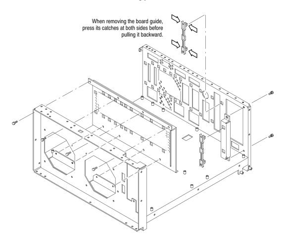
Figure 6-30: Board guide bracket removal
