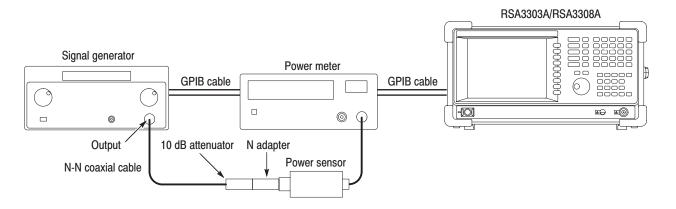
Figure 5-2: Initial test hookup
