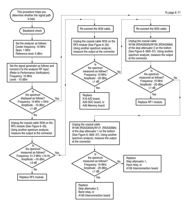
Figure 6-34: Troubleshooting procedure 3 — Signal path
