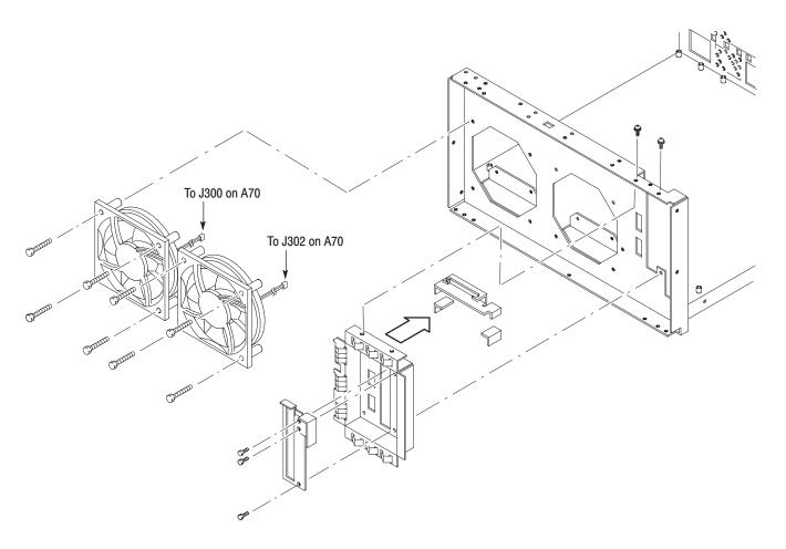
Figure 6-29: Fan and side panel removal
