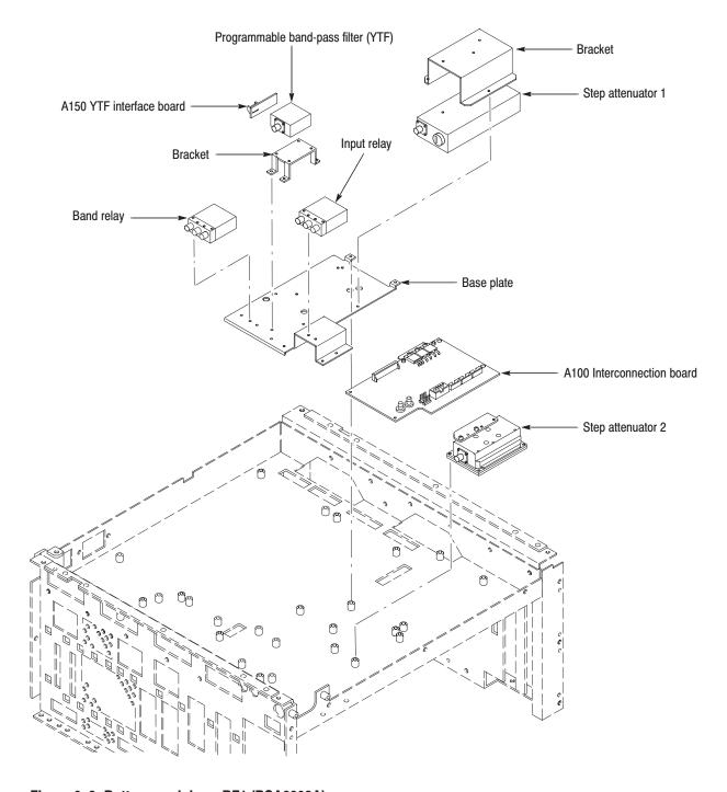
Figure 6-8: Bottom modules - RF1 (RSA3308A)
