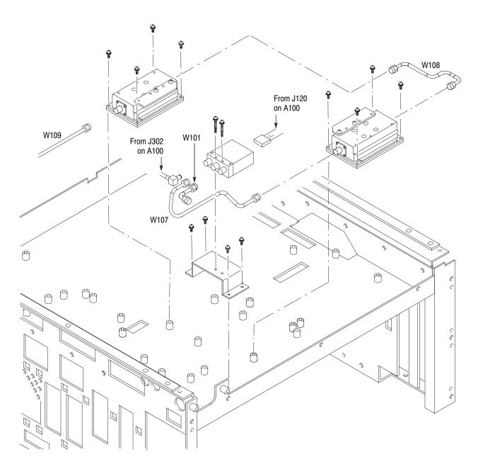
Figure 6-24: RF1 modules removal - 2 (RSA3303A)
