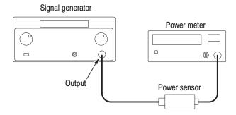
Figure 4-10: Hookup for setting the signal generator output
