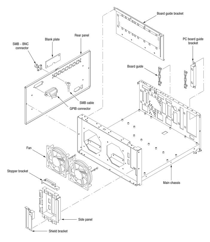
Figure 6-10: Chassis modules
