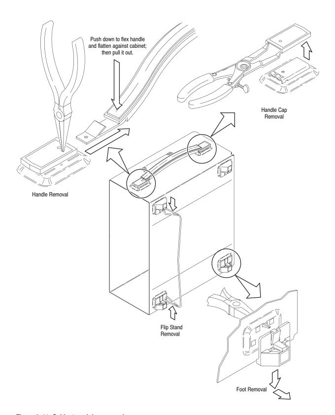
Figure 6-14: Cabinet modules removal
