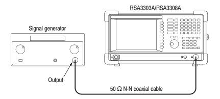
Figure 4–12: Initial test hookup
