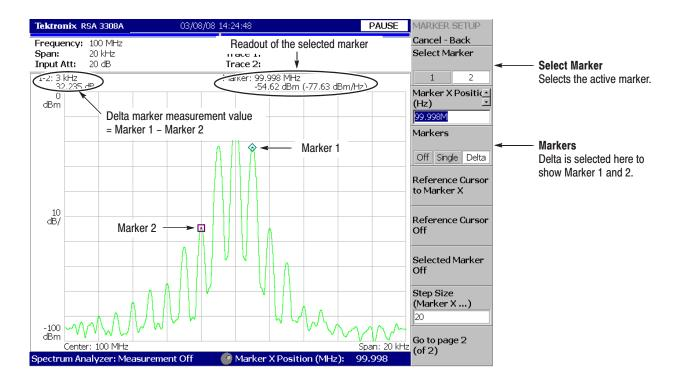
Figure 2-21: Measurement with the delta marker
