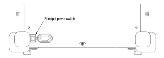
Figure 2-2: Principal power switch (rear panel)
