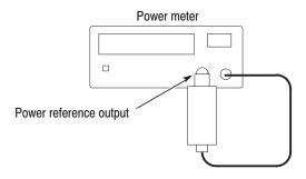
Figure 4-9: Hookup for calibrating the power sensor
