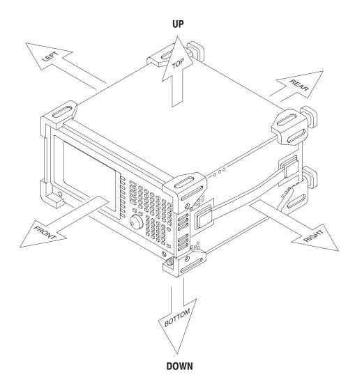
Figure 6-1: Analyzer orientation
