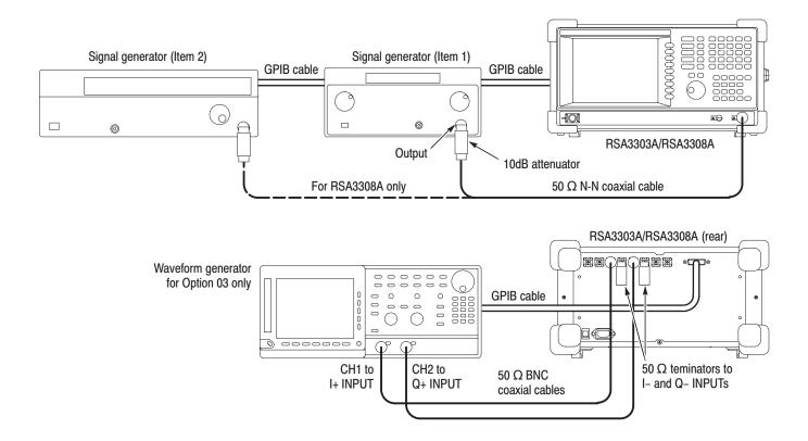
Figure 5-8: Initial test hookup
