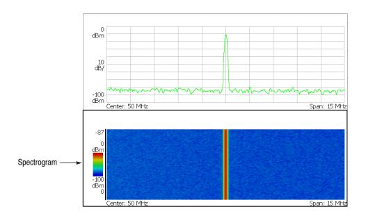
Figure 4-4: Spectrogram display
