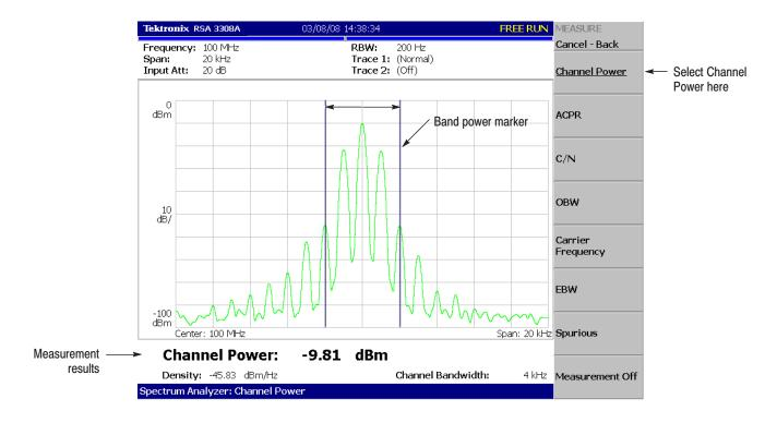
Figure 2-28: Channel power measurement
