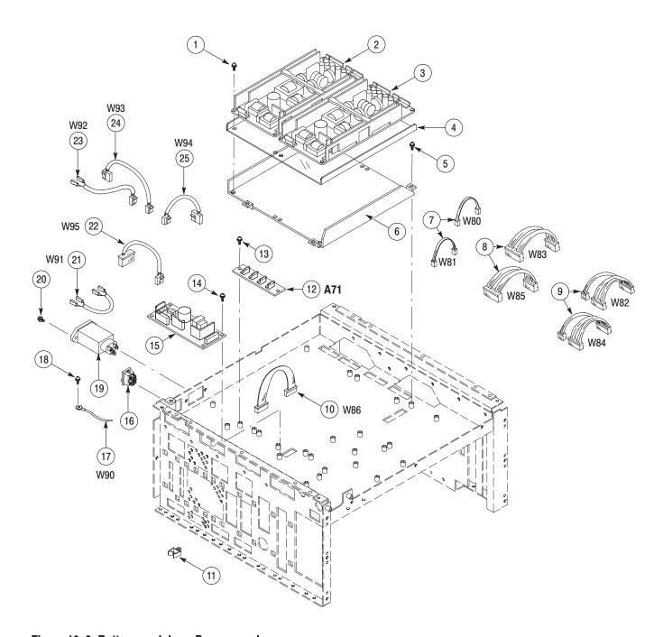
Figure 10-8: Bottom modules - Power supply
