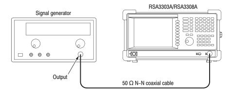
Figure 4-13: Initial test hookup
