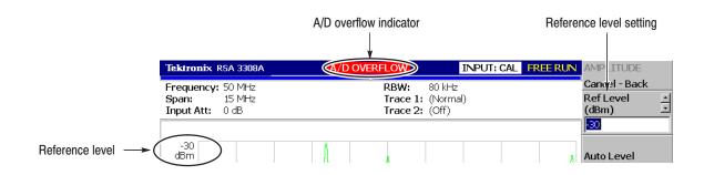
Figure 4-3: Reference level setting and A/D overflow indicator
