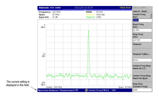
Figure 2-14: Center frequency of 100 MHz, span of 15 MHz
