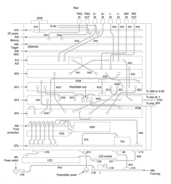
Figure 6-35: Top view for cable interconnection
