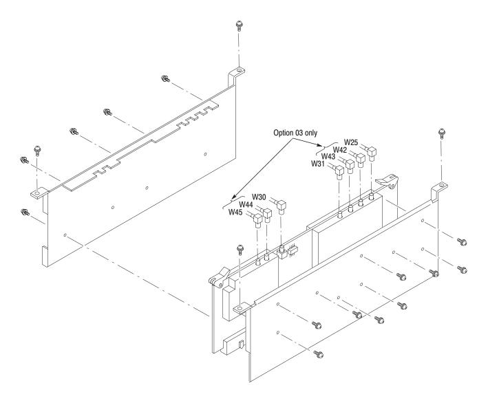
Figure 6-18: A10 A/D board removal
