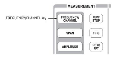
The FREQUENCY/CHANNEL menu, shown in Figure 2–12, is displayed on the right side of the screen. Notice that the Frequency menu item is available for entering the numeric value for center frequency.
