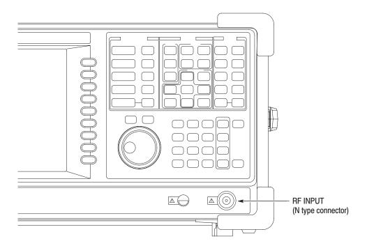
Figure 2-7: Cable connection
