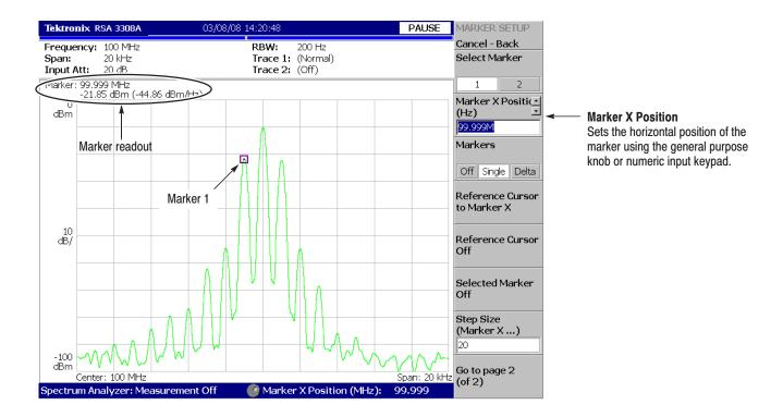
Figure 2-20: Measurement with a single marker
