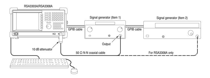
Figure 4-6: Initial test hookup
