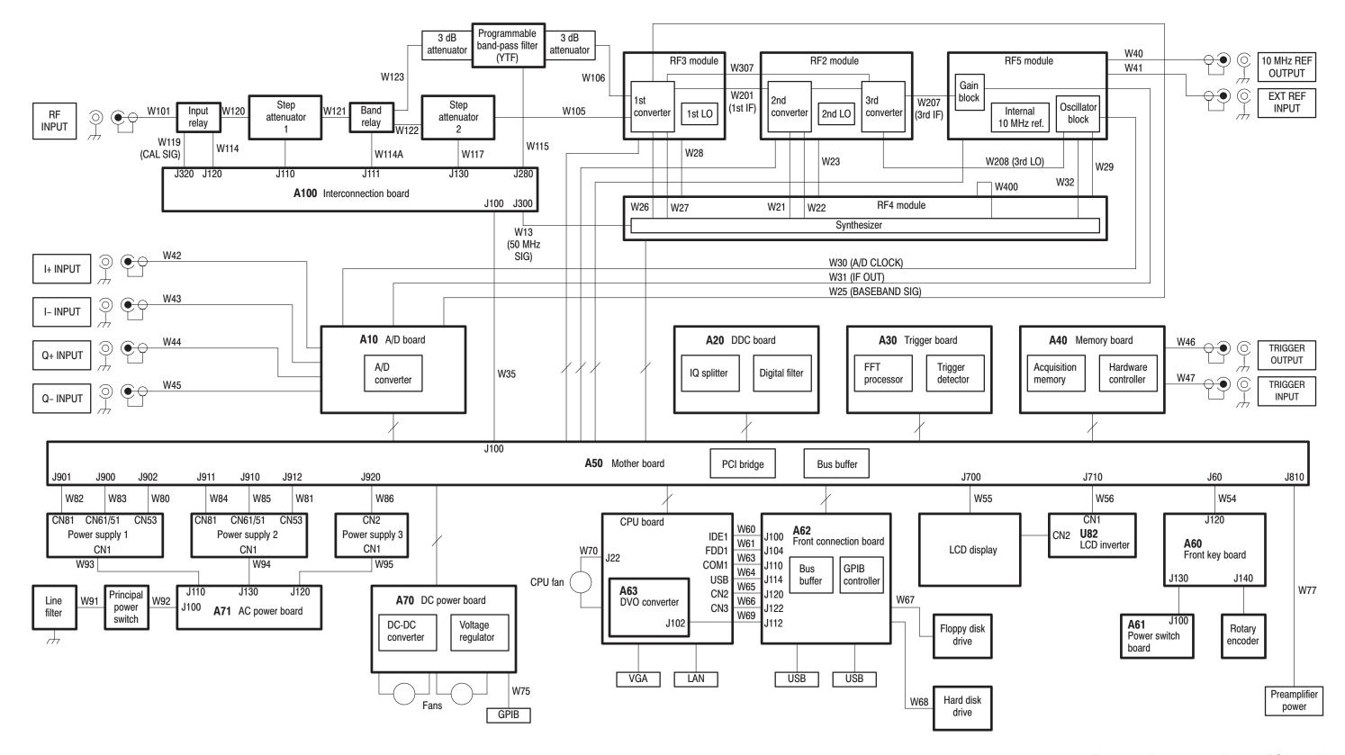
Figure 9-3: Interconnect diagram (RSA3308A)
