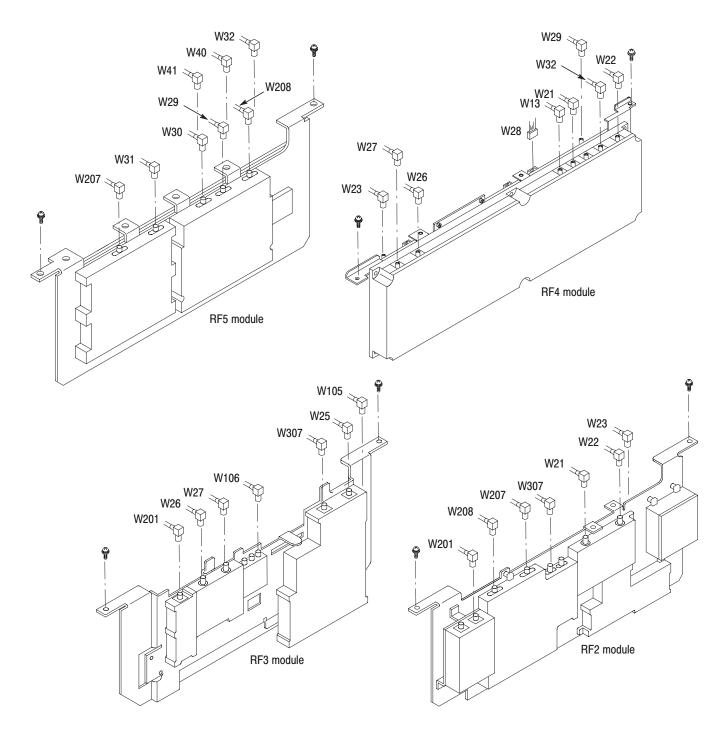
Figure 6-15: RF modules removal
