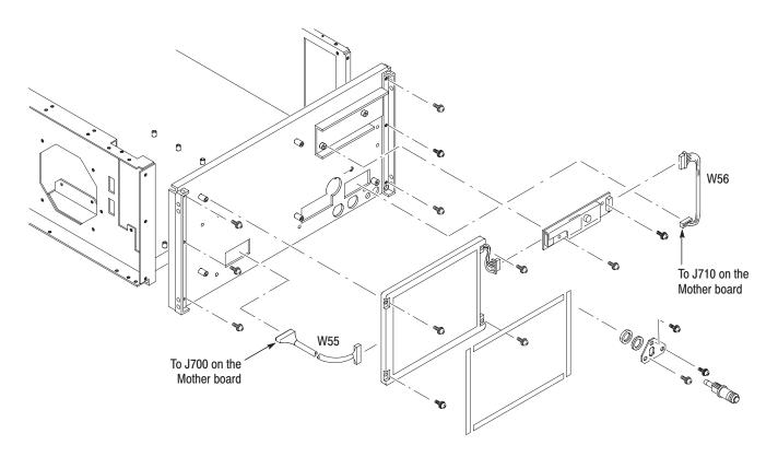
Figure 6-28: LCD display removal
