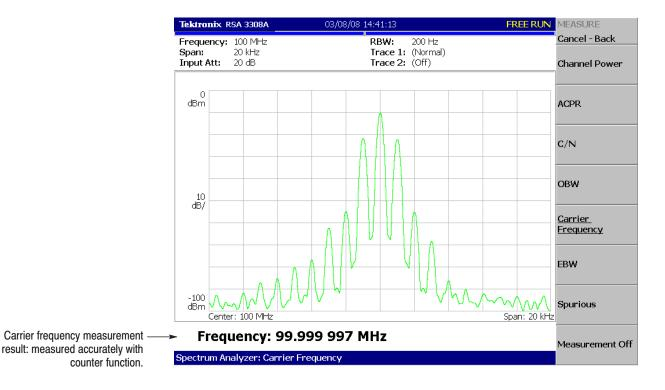
Figure 2-30: Carrier frequency measurement
