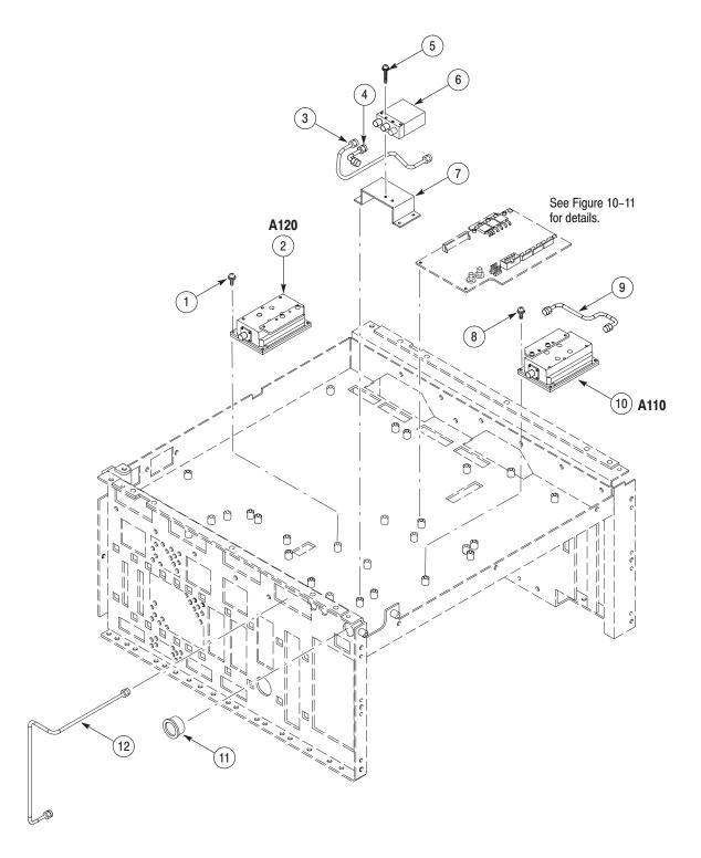
Figure 10-9: Bottom modules - RF1 (RSA3303A)
