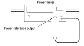
Figure 5–3: Hookup for calibrating the power sensor
