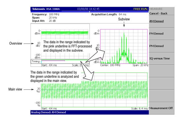
Figure 2-32: AM signal measurement
