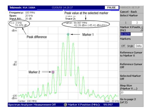
The difference between the two marker positions is shown in the upper left part of the screen (see Figure 2–22).
