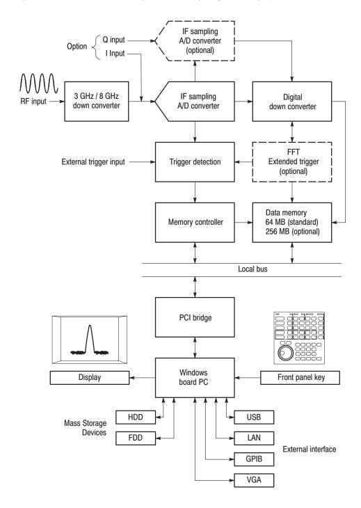
Figure 1-6: Block diagram
