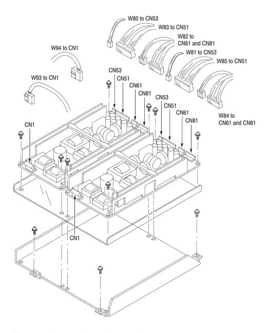
Figure 6-21: Power supply 1 and 2 removal
