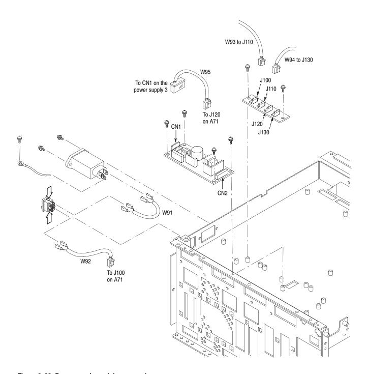
Figure 6-22: Power supply modules removal
