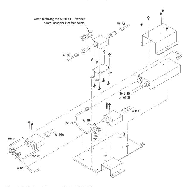
Figure 6-25: RF1 modules removal - 2 (RSA3308A)
