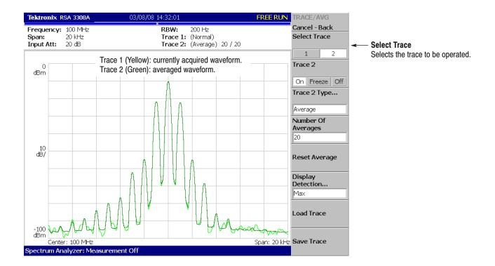
Figure 2-24: Comparison display with averaged waveform
