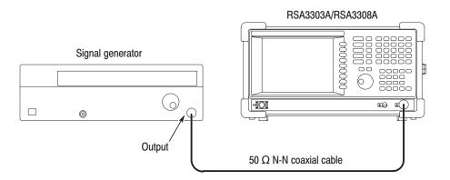
Figure 4-14: Initial test hookup
