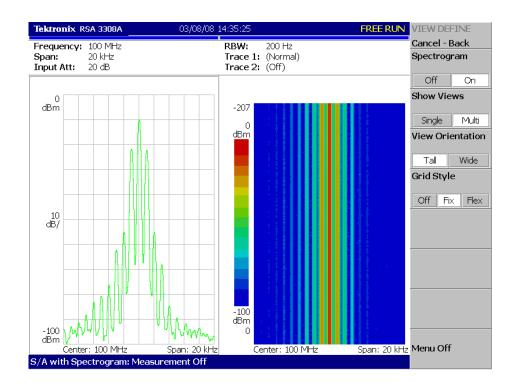
Figure 2-26: Tall display of spectrum and spectrogram
