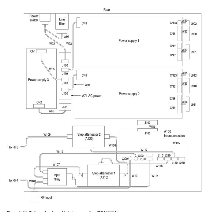
Figure 6-36: Bottom view for cable interconnection (RSA3303A)
