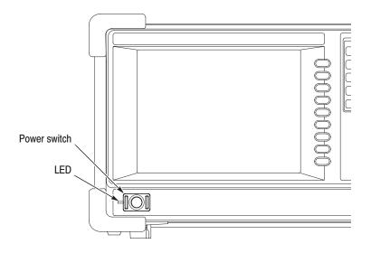
Figure 2-9: Power switch (ON/STANDBY)
