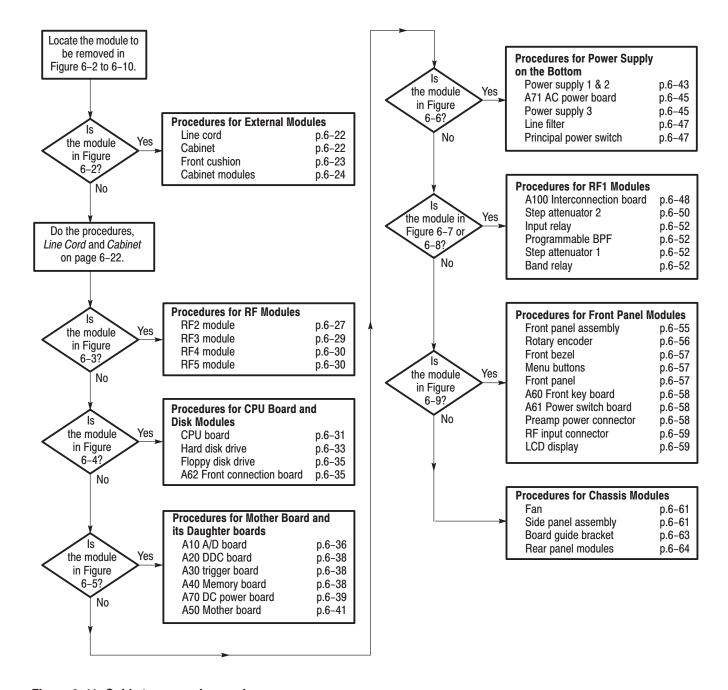
Figure 6-11: Guide to removal procedures
