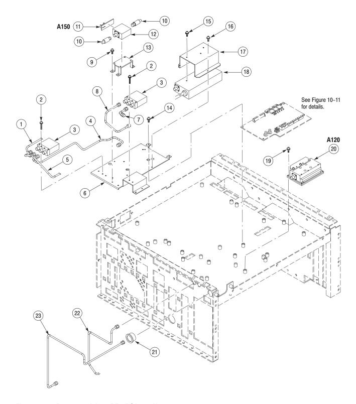
Figure 10-10: Bottom modules - RF1 (RSA3308A)
