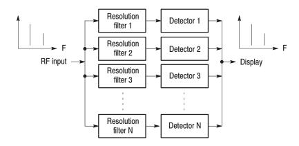
Figure 1-3: Concept of the real-time spectrum analyzer
