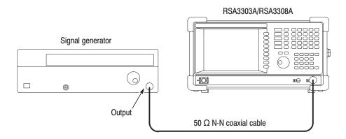
Figure 4-15: Initial test hookup
