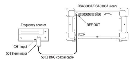
Figure 5-9: Initial test hookup
