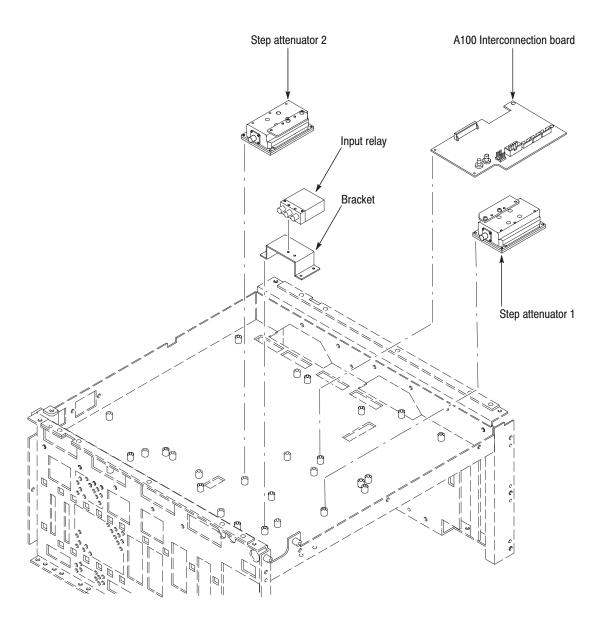
Figure 6-7: Bottom modules - RF1 (RSA3303A)
