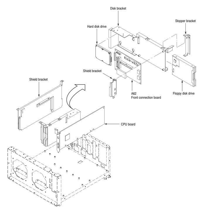
Figure 6-4: CPU board and disk modules
