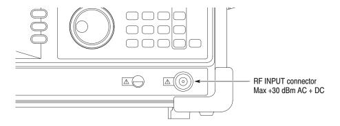
Figure 2-5: RF INPUT connector
