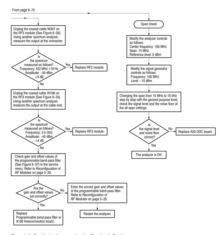
Figure 6-34: Troubleshooting procedure 3 — Signal path (Cont.)
