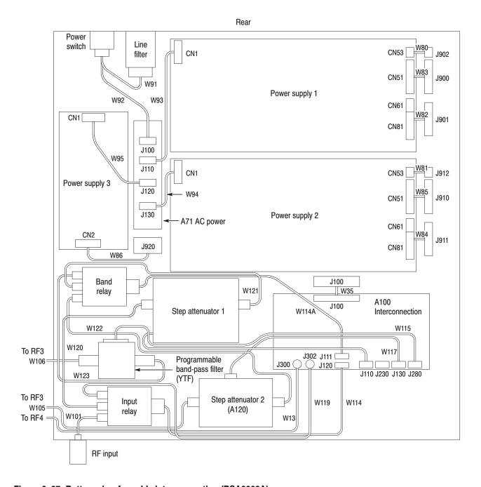
Figure 6-37: Bottom view for cable interconnection (RSA3308A)
