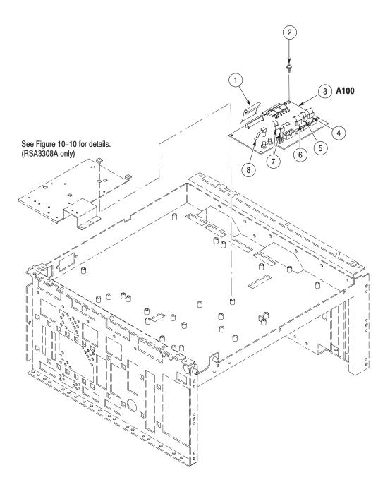
Figure 10-11: Bottom modules - Interconnection
