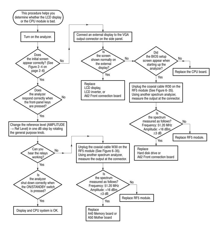
Figure 6-33: Troubleshooting procedure 2 — Display and CPU system
