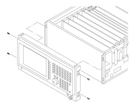
Figure 6-26: Front panel assembly removal
