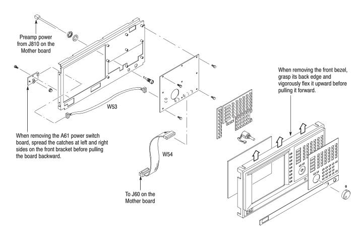
Figure 6-27: Front panel modules removal
