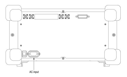
Figure 2-1: AC Input (rear panel)
