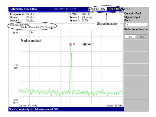
Figure 4-1: Spectrum of the calibration signal (50 MHz, -20 dBm)
