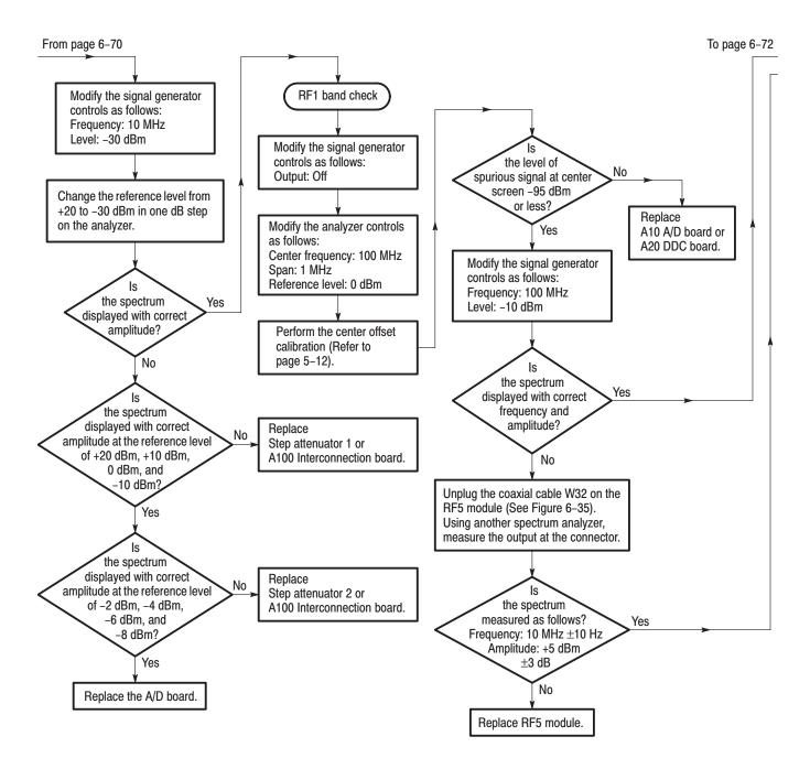
Figure 6-34: Troubleshooting procedure 3 — Signal path (Cont.)
