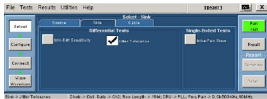
3. To change the configuration settings, click **Tests > Configure**. For most tests, you can use the factory default configuration. However, you can change the values by using the virtual keyboard or the general purpose knob on the oscilloscope front panel. Using the File menu, you can also restore the factory defaults or save and recall your own configuration settings.
