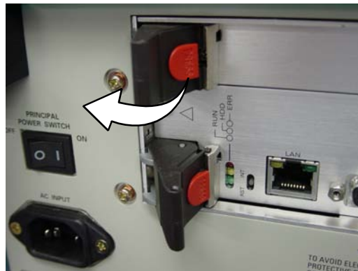
Figure 6-9: CD-ROM module removal
