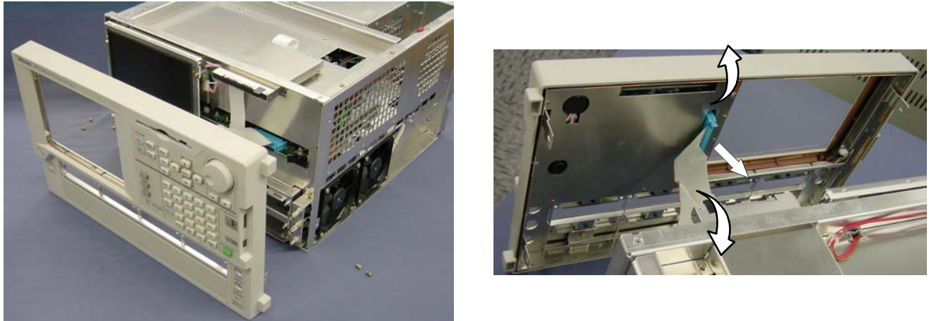
Figure 6-16: Front-Panel assembly removal
