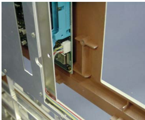
Figure 6-18: Front-panel chassis removal
