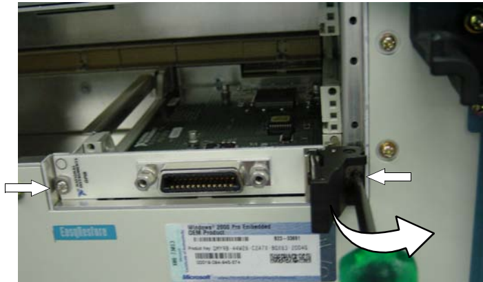
Figure 6-12: Loosen the screws
