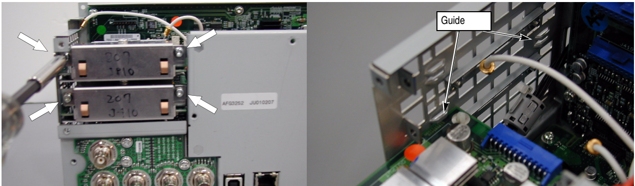
Figure 6-9: Output board removal
