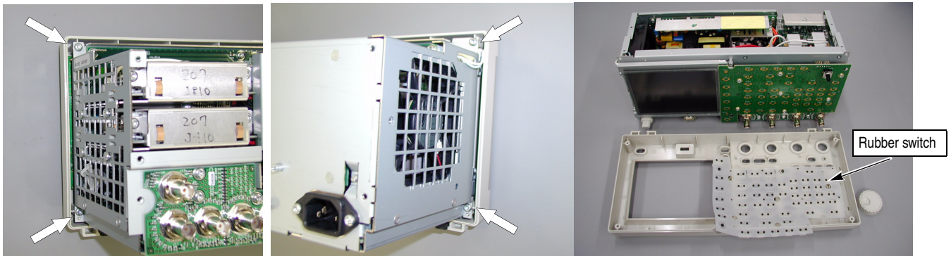
Figure 6-6: Front case removal
