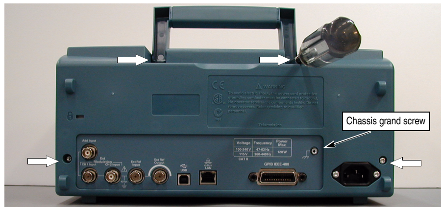
Figure 6-3: Rear case removal
