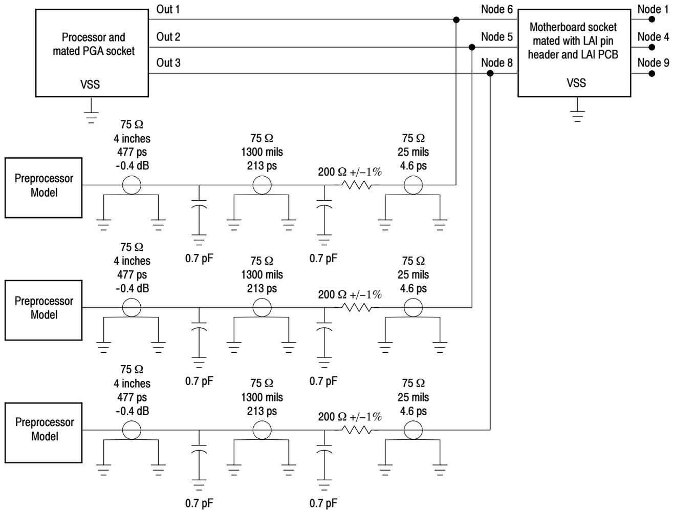
Figure 9: Probe adapter load model for typical signals
