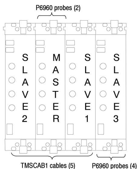
**Figure 2: Module configuration**
