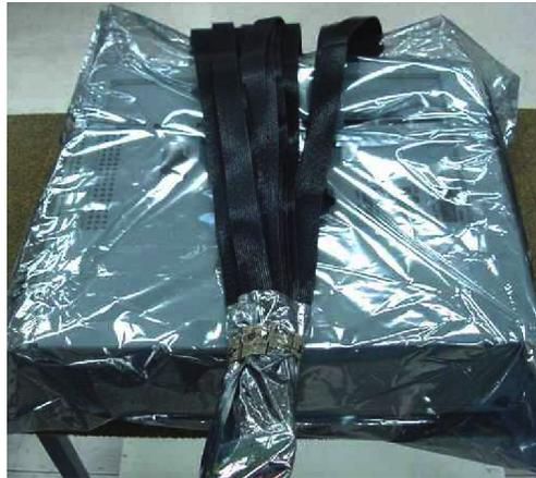
**Figure 6: Preprocessor unit in static-shielding bags**
