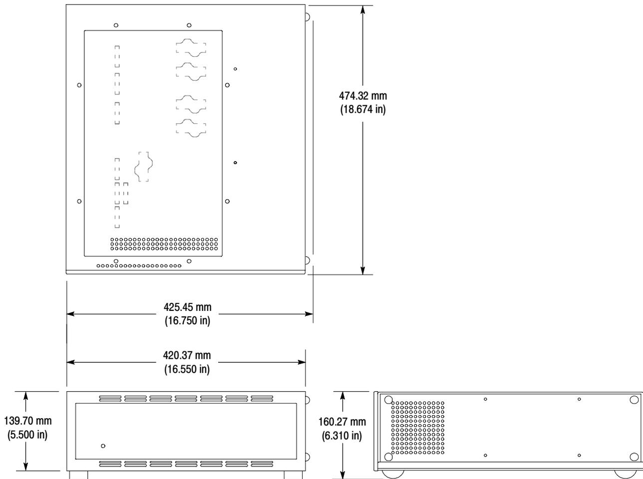
**Figure 16: Dimensions of the preprocessor unit**
