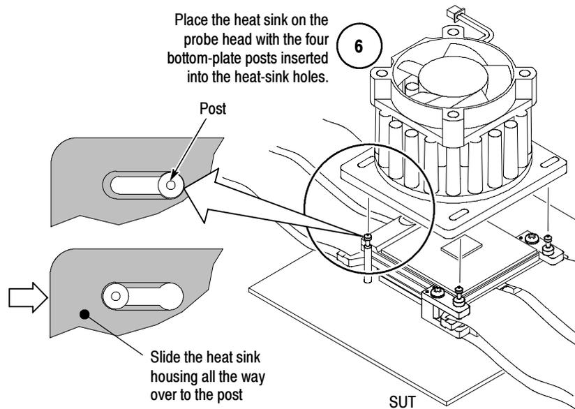
**Figure 5: Install heat sink (Chipcool 1 & 2)**
