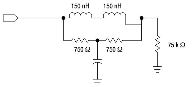
**Figure 13: Receiver topology C**
