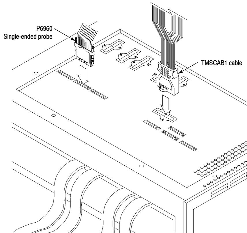
**Figure 3: Probe, cable and preprocessor unit**
