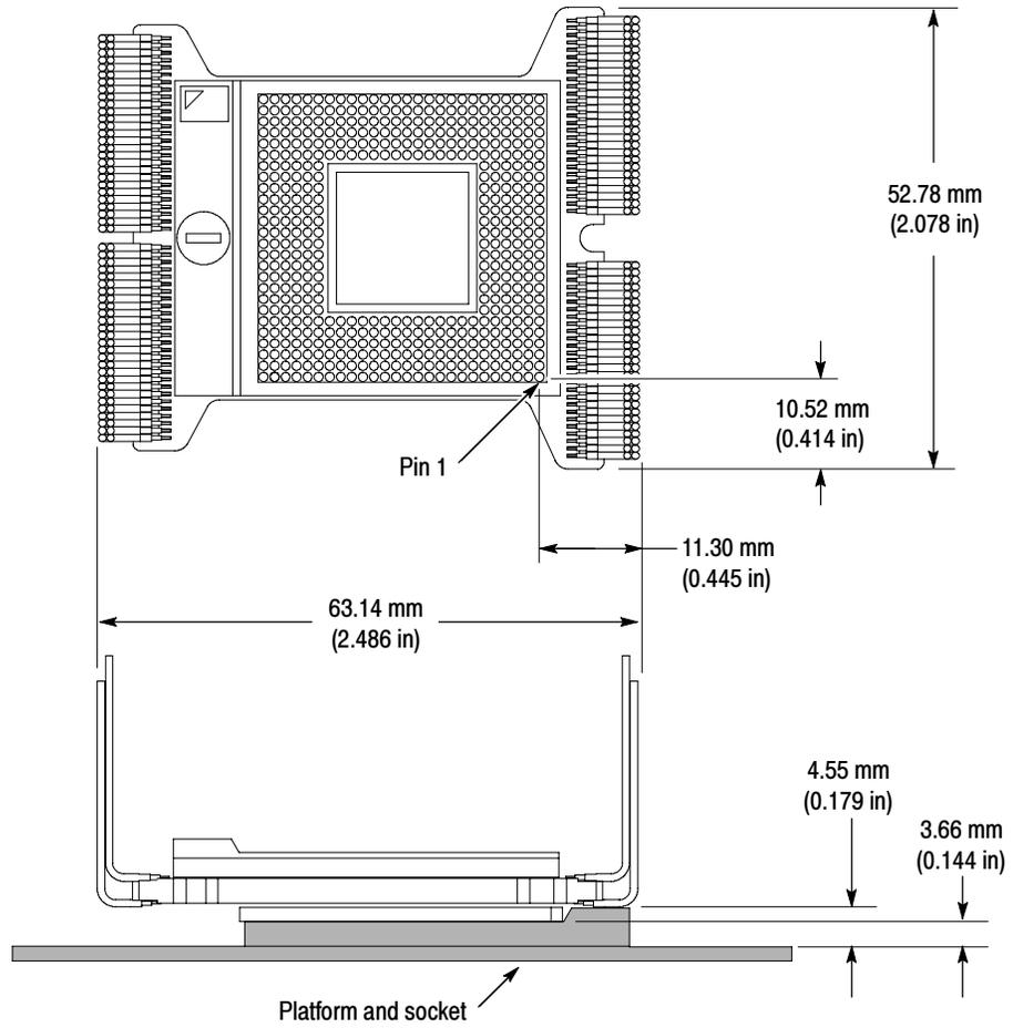
**Figure 15: Dimensions of the probe head**
