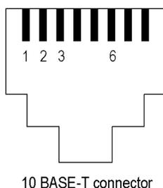
**Table 2-3: Pin assignments of the 10 BASE-T connector for the mainframe GPI**
