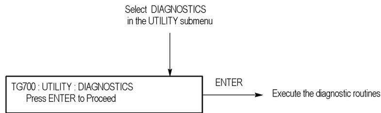
**Figure 2-24: DIAGNOSTICS submenu**
