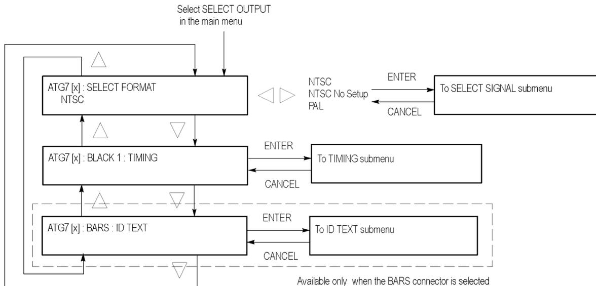
**Figure 3-11: ATG7 module SELECT OUTPUT submenu**
