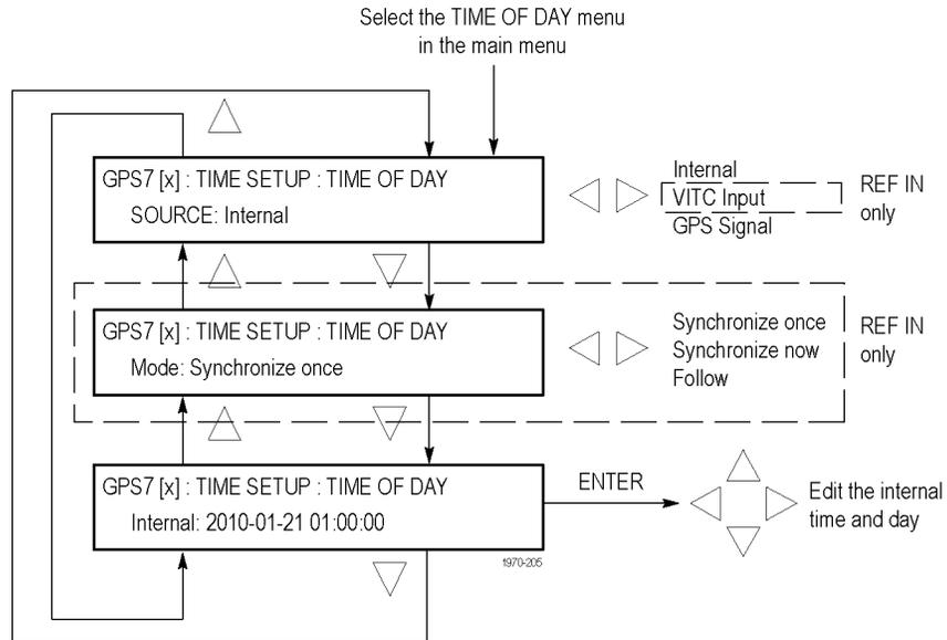
**Figure 3-62: GPS7 module TIME OF DAY submenu**
