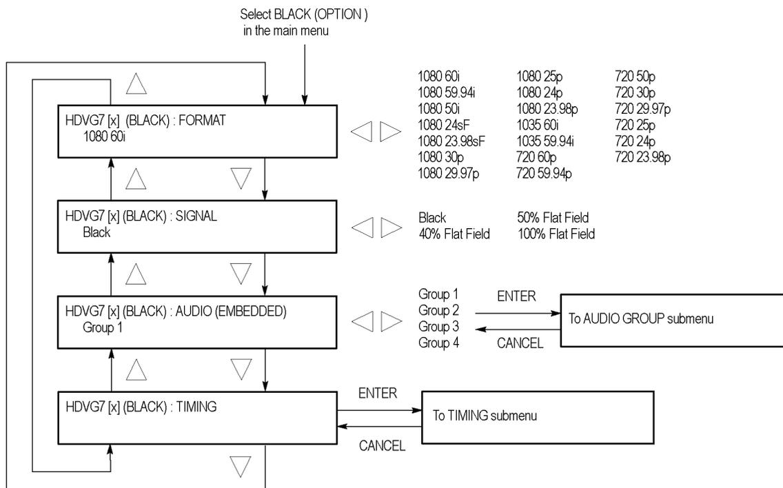
Figure 3-112: HDVG7 module BLACK submenu (Option BK only)
