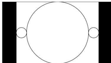
Figure 3-93: AFD code '1001' for a 16:9 coded frame
