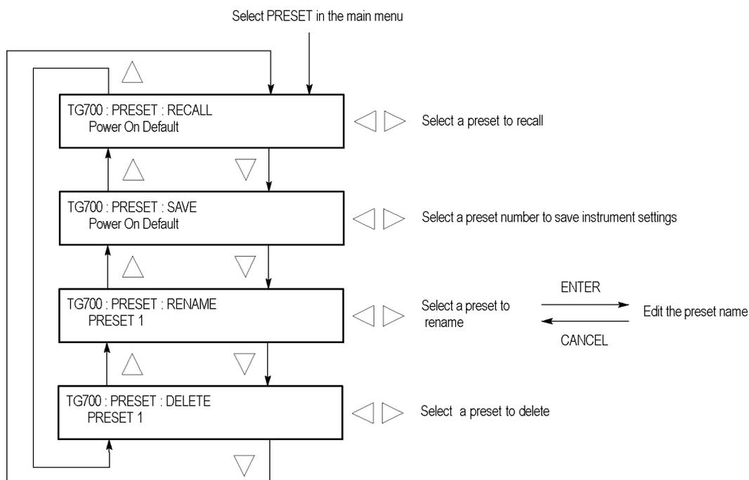
Figure 2-17: PRESET submenu
