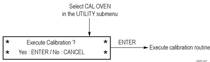
**Figure 2-25: Internal frequency calibration menu**
