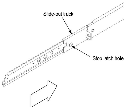
**Figure 1-2: Placing the TG700 in the rack**
