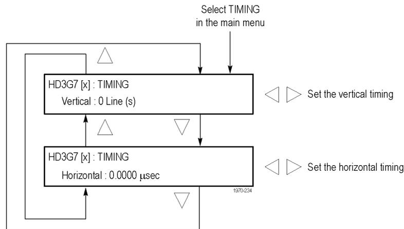
**Figure 3-88: HD3G7 module TIMING submenu**
