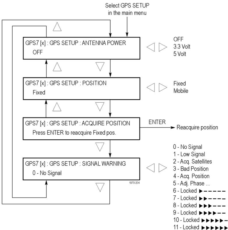
**Figure 3-61: GPS7 module GPS SETUP submenu**
