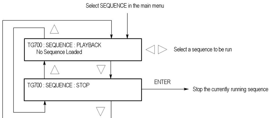
**Figure 2-18: SEQUENCE submenu**
