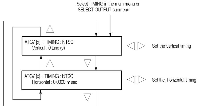
**Figure 3-14: ATG7 module TIMING submenu**
