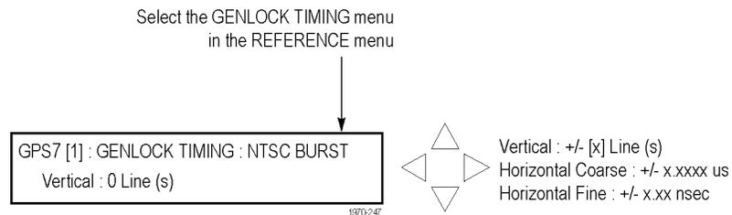
Use the up (▲) or down (▼) arrow button to select a timing parameter, and then use the left (◀) or right (▶) arrow button to adjust the parameter.
