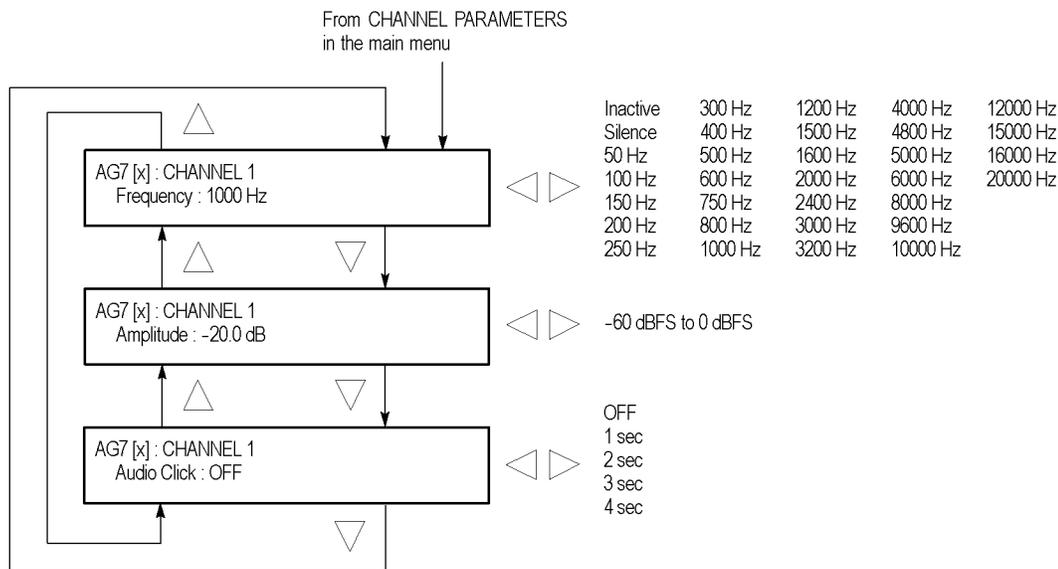
Figure 3-2: AG7 module CHANNEL PARAMETERS submenu
