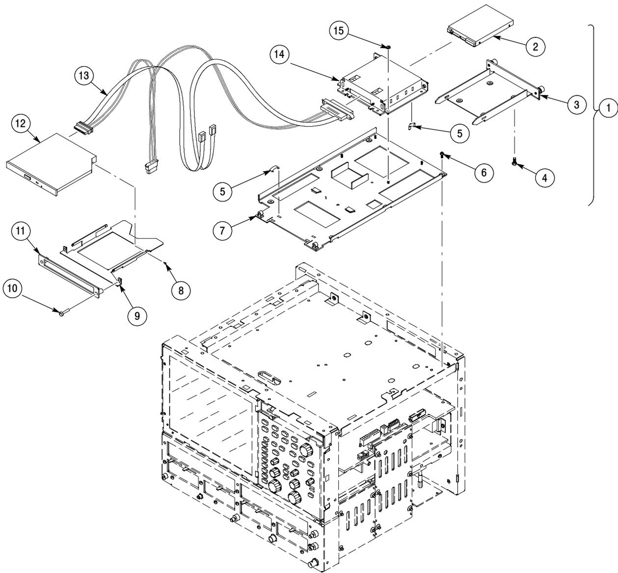
Figure 6-2: Drives (SN B03000 and above)
