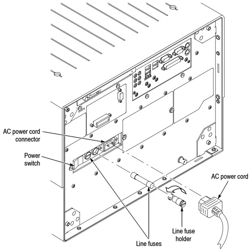
**Figure 4-1: Line fuses and line cord removal**
