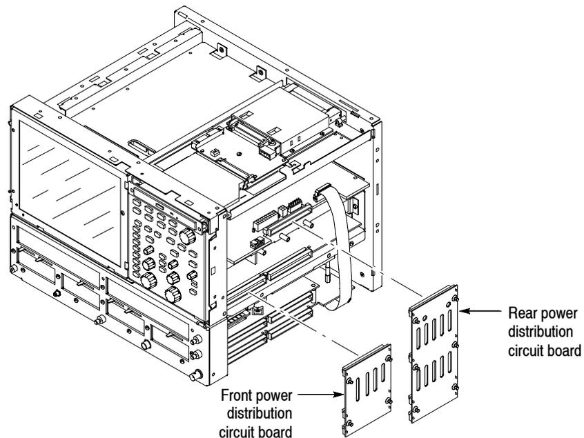
**Figure 4-33: Front and rear power distribution board removal**
