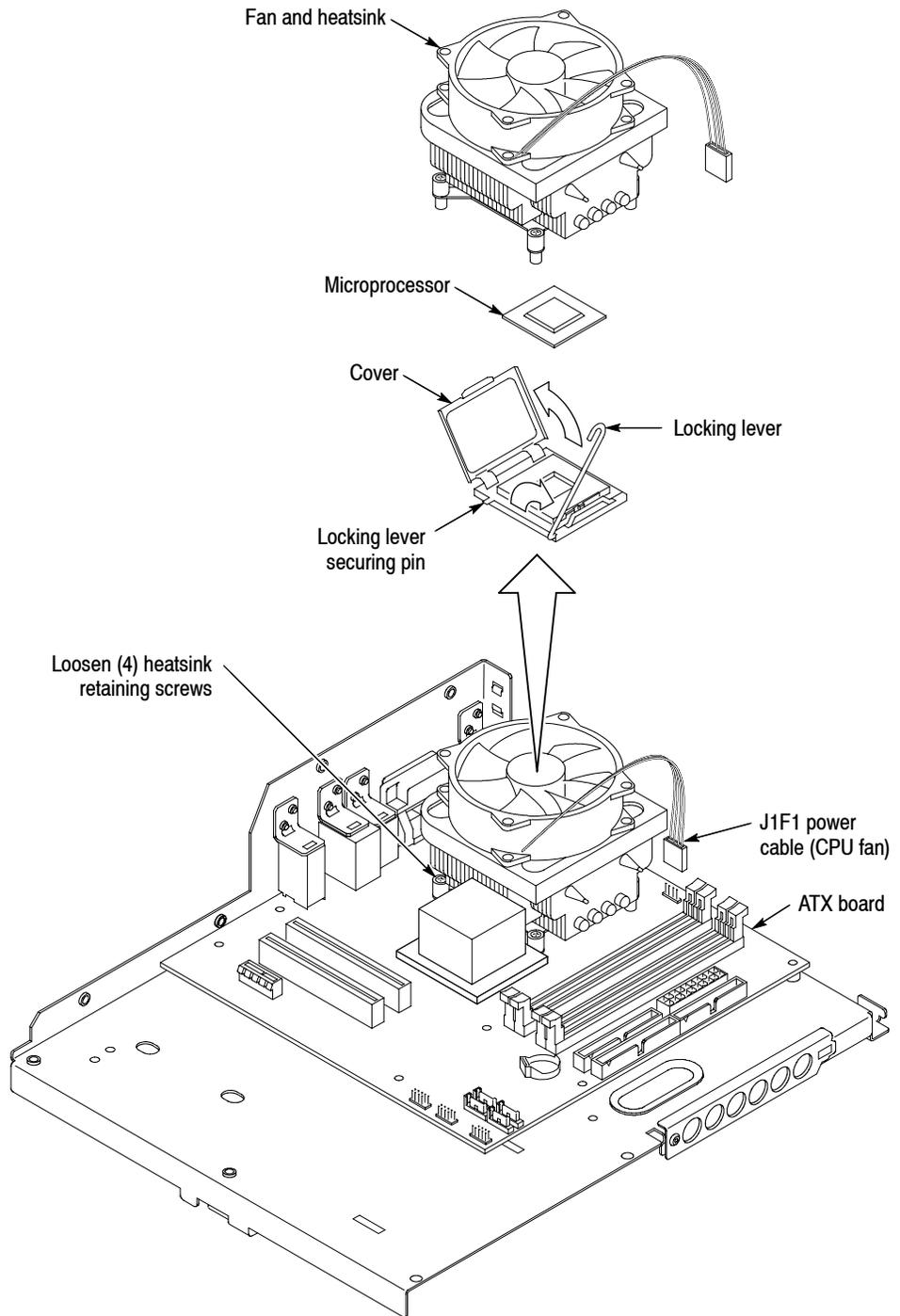
**Figure 4-32: Microprocessor removal**
