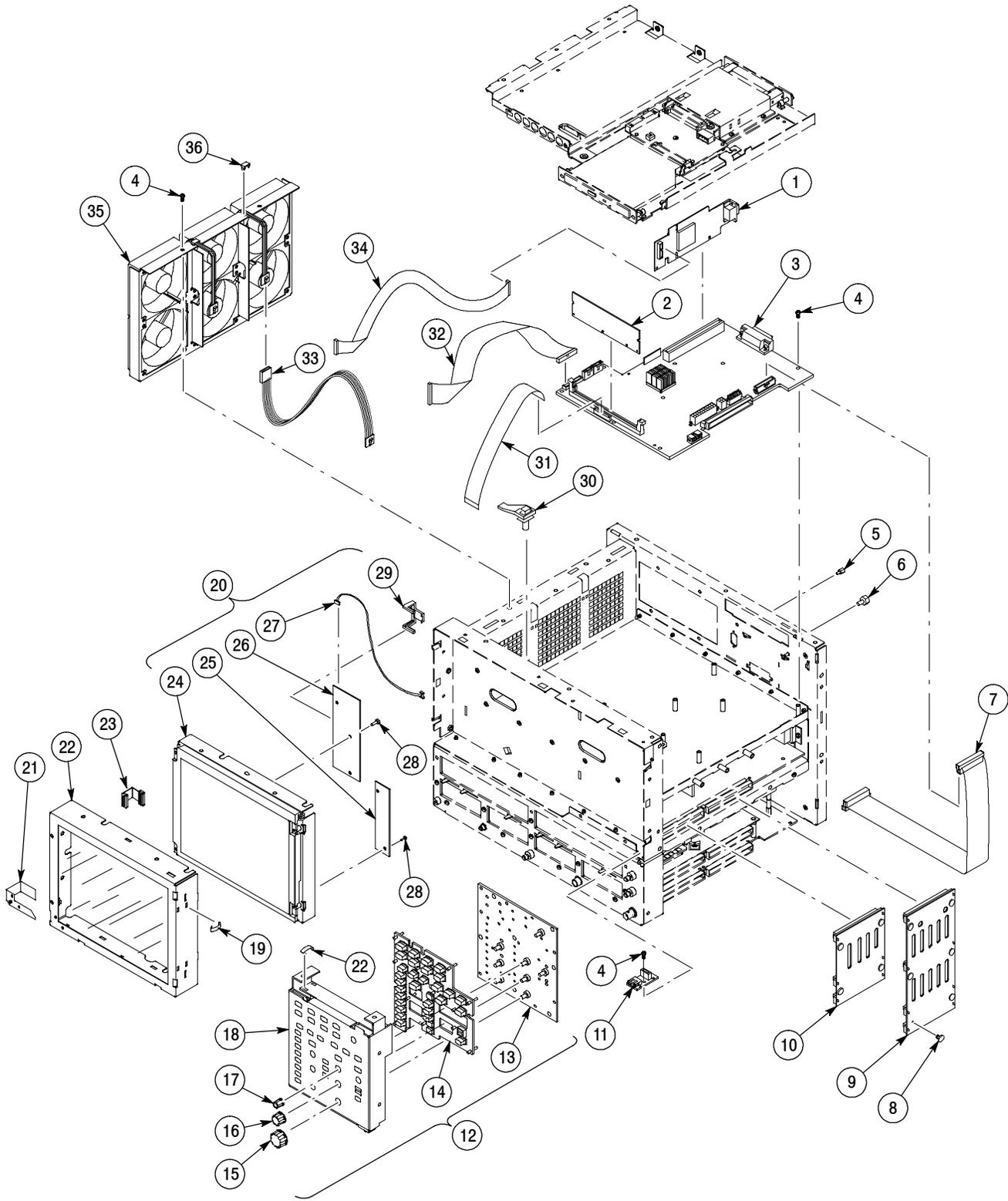
**Figure 6-4: Front panel and processors**
