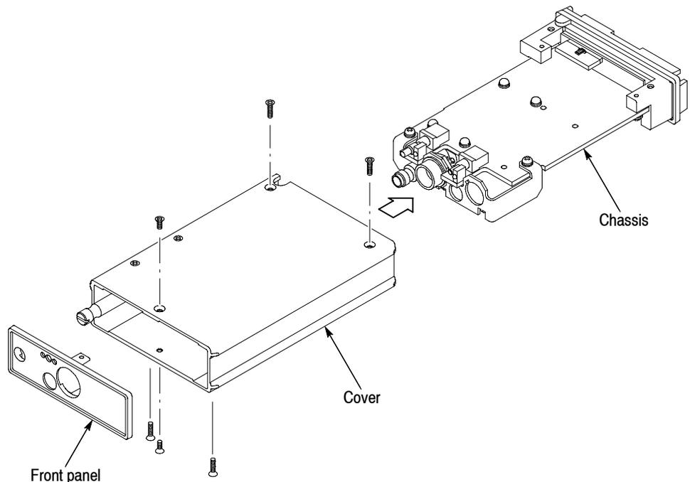
**Figure 4-46: Sample of electrical module hardware removal**
