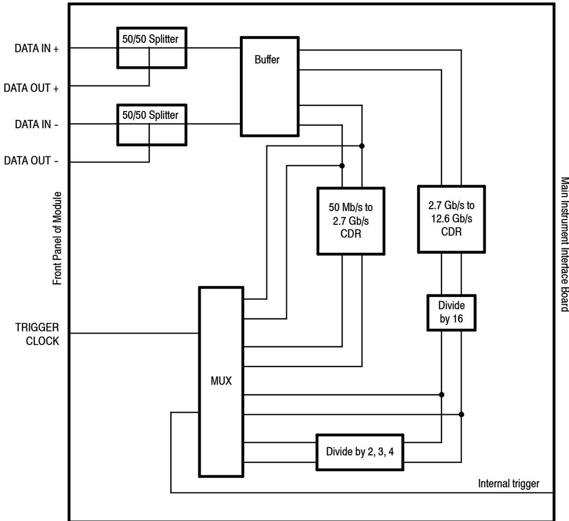
Figure 5-5: 80A05 block diagram
