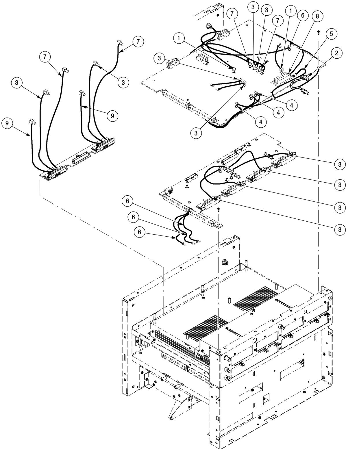
Figure 6-9: Coaxial cables
