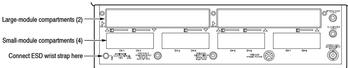
**Figure 1-1: Compartments for sampling modules**
