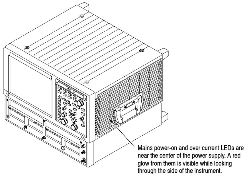
**Figure 4-49: Location of power-on and over current LEDs**
