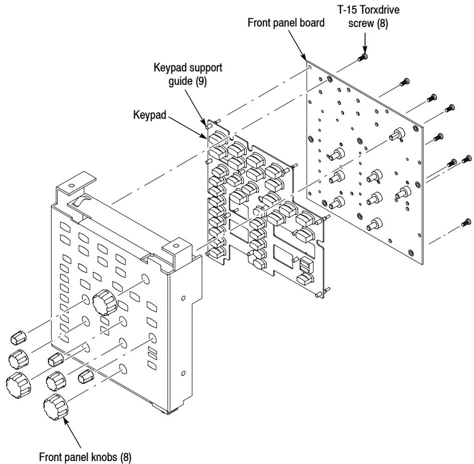
**Figure 4-12: Front panel board and keyboard removal**
