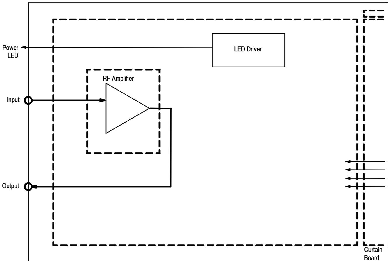
Figure 5- 3: 80A01 block diagram
