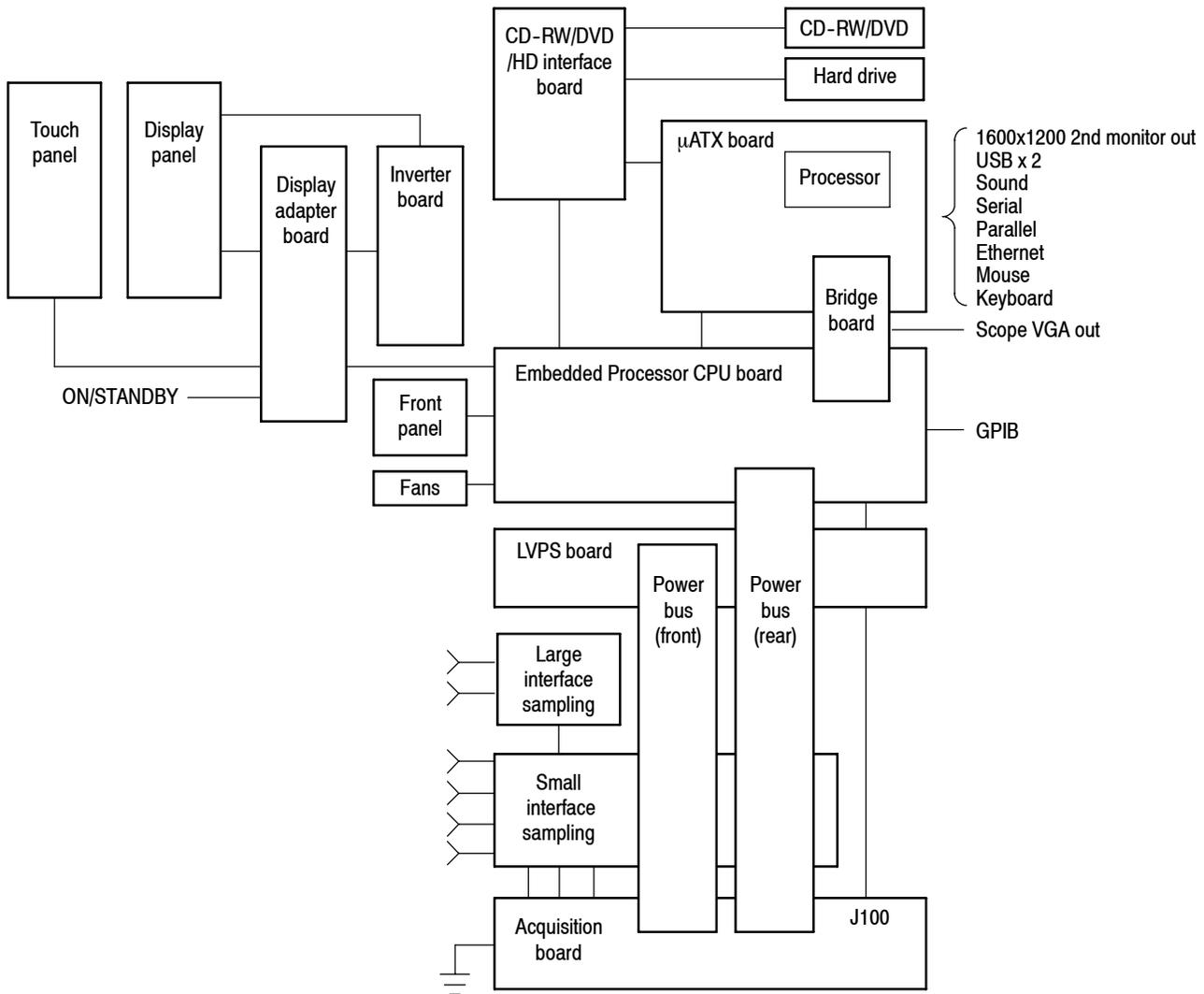
Figure 5- 1: Block diagram for the DSA8200
