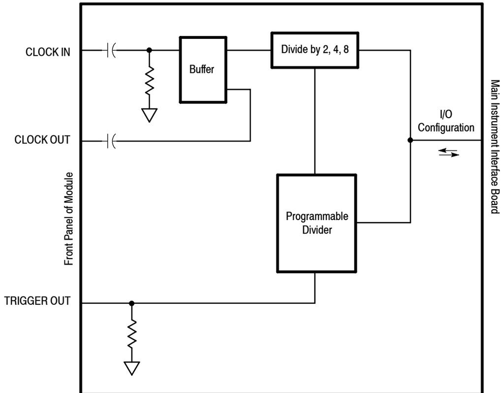
Figure 5-6: 80A06 block diagram
