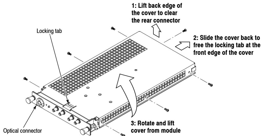
**Figure 4-47: Optical module cover removal**
