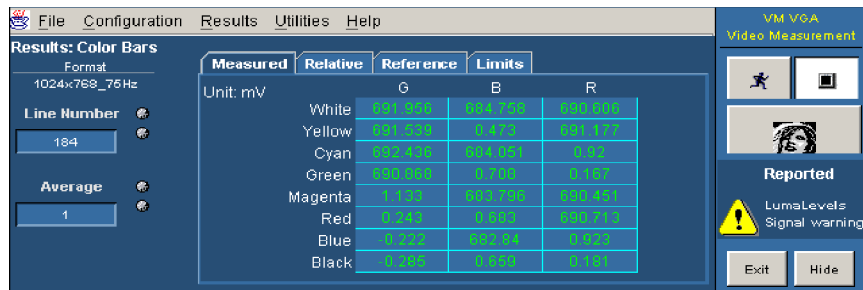
Figure 3-63: Color Bars measurement results
