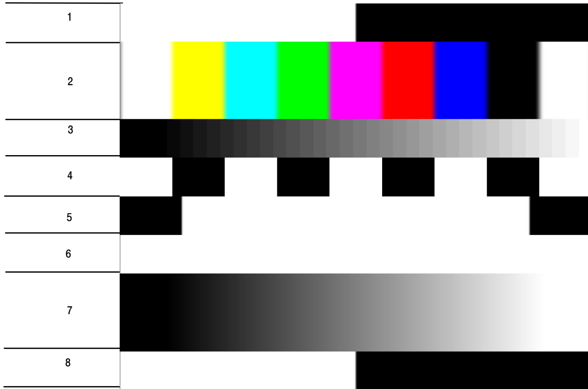
Figure 2-33: Option VGA Matrix test signal
