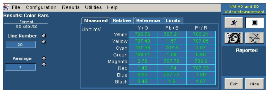
Figure 3-28: Displaying the Color Bars measurement
