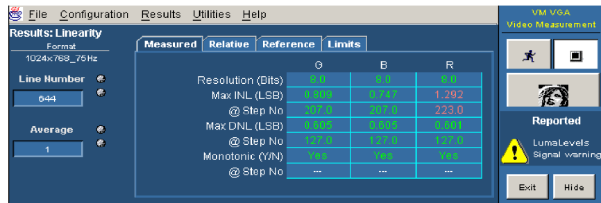
Figure 3-71: Linearity measurement results
