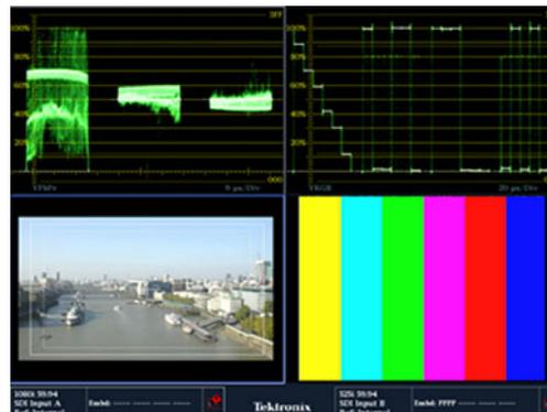
**NOTE.** The status bar at the bottom of the screen shows which side of the display is associated with which link.
