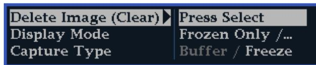
3. Press **SEL** to delete the frozen image. The pop-up menu is automatically removed from the display when the frozen image is deleted.
