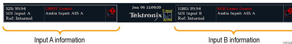
Figure 2: Status bar in simultaneous input mode
