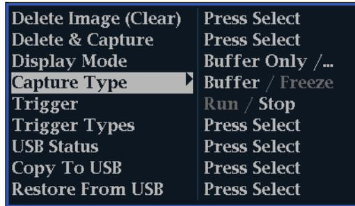
**NOTE.** The capture type chosen is specific to the tile selected for FREEZE, but is universal for BUFFER.
