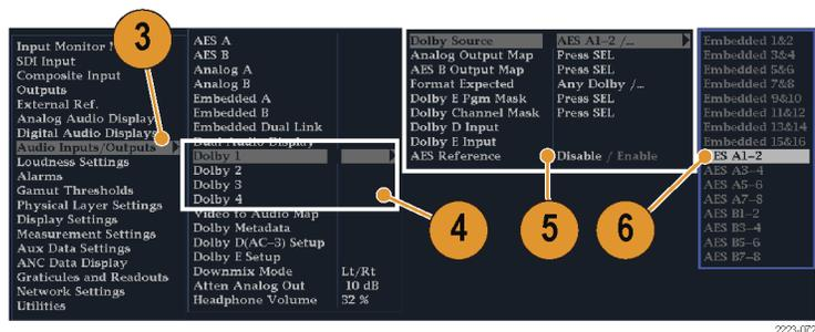
7. Select **Format Expected** and choose the format condition that, when missing, triggers the Dolby Format Alarm.
