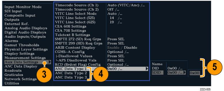
**NOTE.** If the Name is left blank and you select a DID and SDID, then the name of the ANC data type will be filled in automatically on the Aux Data Status display.
