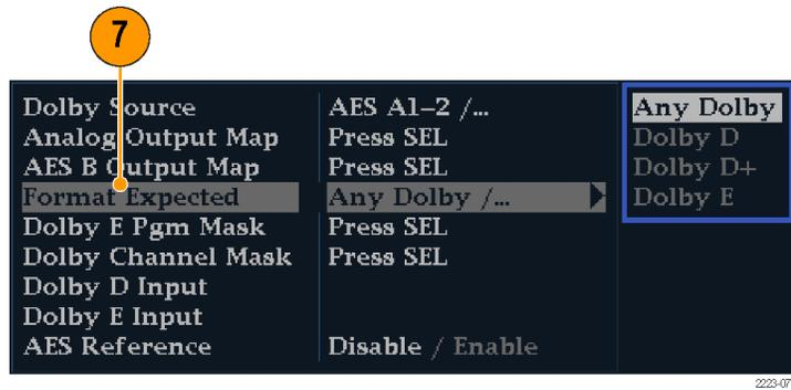
8. Select **Analog Output Map** and specify which inputs (if any) are routed to the analog outputs in the map that appears. (Map shown right.)
