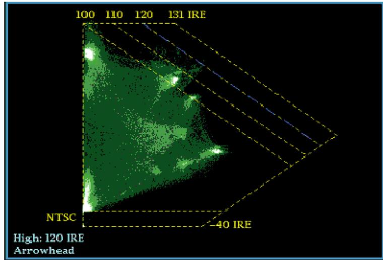
Another useful Arrowhead function is a measure of how well the active video signal is using the dynamic range of the video channel. A properly adjusted signal should be centered in the arrowhead graticule and have transitions that approach all the limits.
