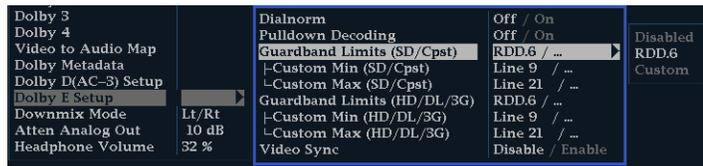
**NOTE.** Dolby E Guardband allows you to set the Dolby E frame location threshold. You can disable the alarm, customize the threshold, or set it to RDD.6, which sets the threshold limits to correspond to the limits in SMPTE RDD.6
