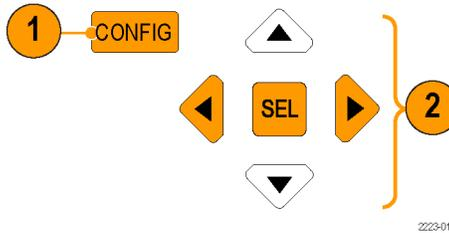
3. Use the up/down arrow keys to move to each the alarm that you want to set. Press **SEL** button to toggle the alarm on (X) or off.
