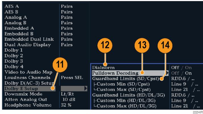
14. Select **Guardband Limits** for either SD/Cpst or HD/DL/3G. If you select **Custom**, you can then set the line maximum and minimum.
