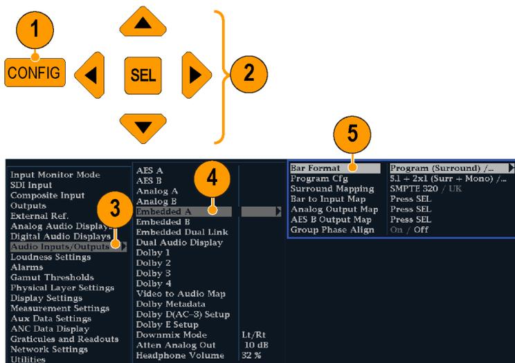
6. Select **Bar to Input Map** and specify which input pair should be displayed in each bar pair.
