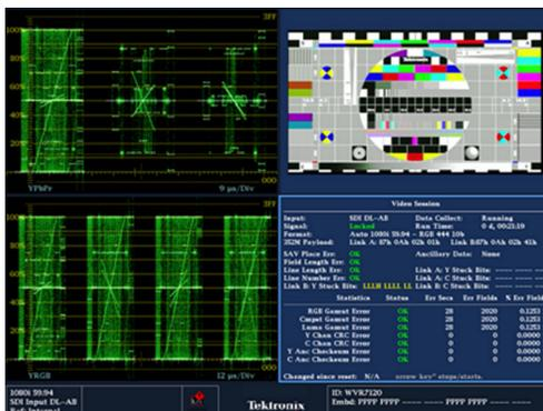
Your instrument will automatically detect the format on signals with SMPTE352M (VPID) while operating on dual link signals. You can then view combined Link A, Link B, and Alpha Channel information, which can help with the identification of correct content. Alpha Channel information will be visible, if present. The next image illustrates where this information appears in the waveform.
