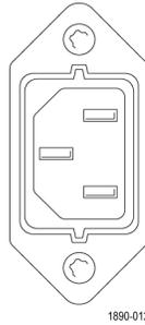
**NOTE.** Only the line conductor is fused for over-current protection. The fuse is internal.
