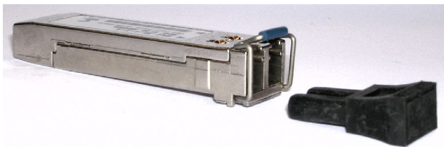
Figure 5: SFP module and optical port plug
