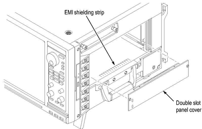
**Figure 4: Installing panel covers on the portable mainframe**
