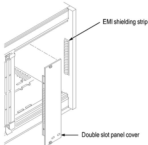
**Figure 5: Installing panel covers on the benchtop mainframe**
