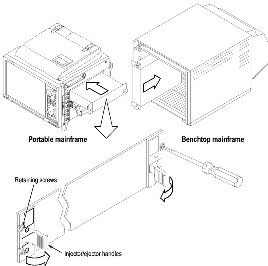
Figure 3: Installing modules
