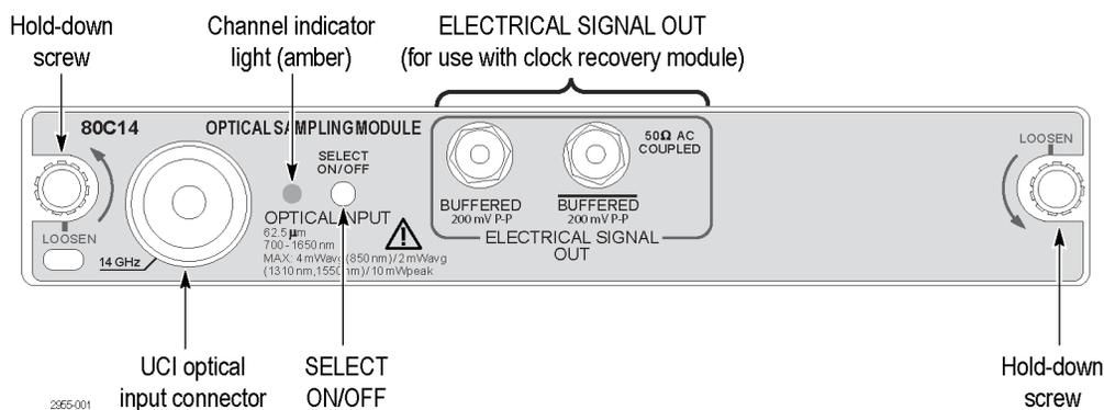
Figure 3: 80C14 optical module front panel
