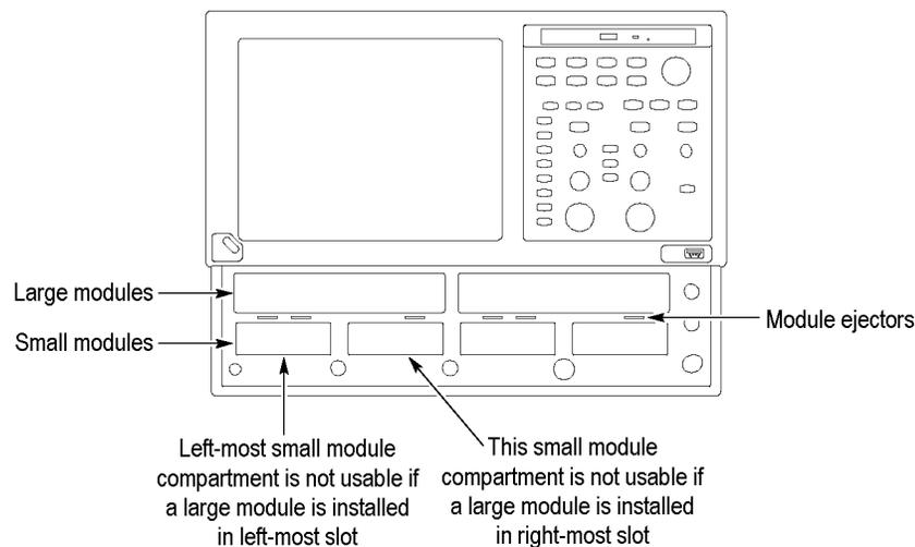
**Figure 1: Module compartments**
