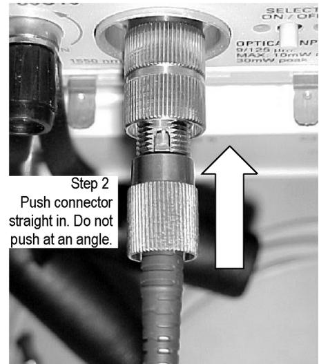
**Figure 2: Connecting optical cables correctly**
