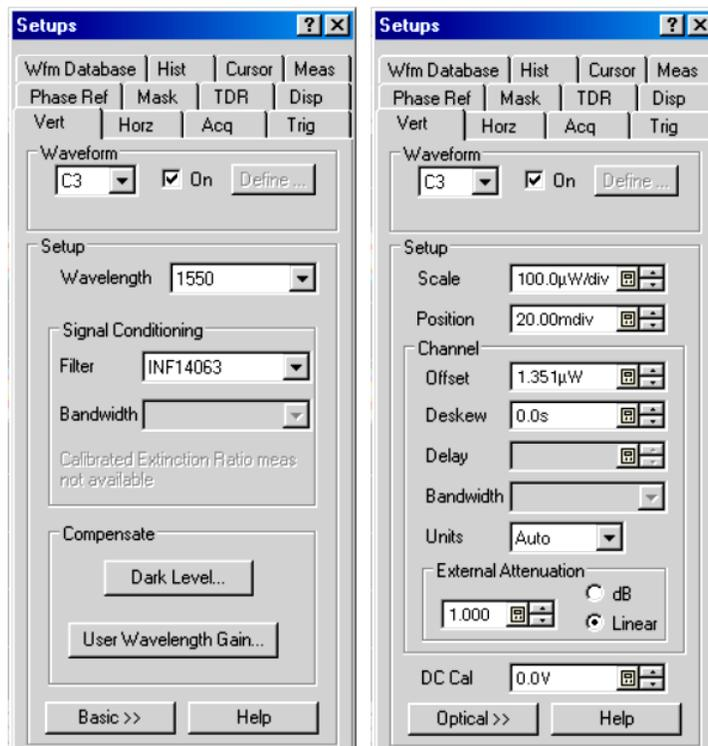
Figure 4: Vertical Setup dialog boxes (DSA8200)
