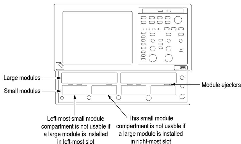
**Figure 1: Module compartments**
