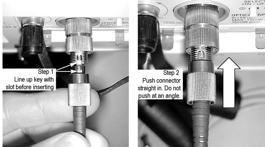
**Figure 2: Connecting optical cables correctly**
