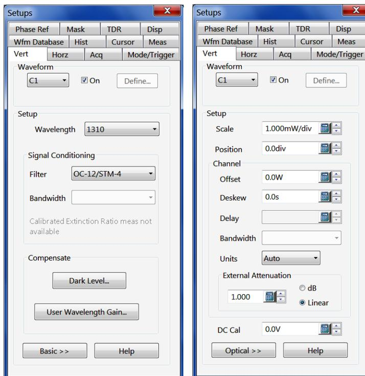
Figure 4: Vertical Setup dialog boxes (DSA8300)
