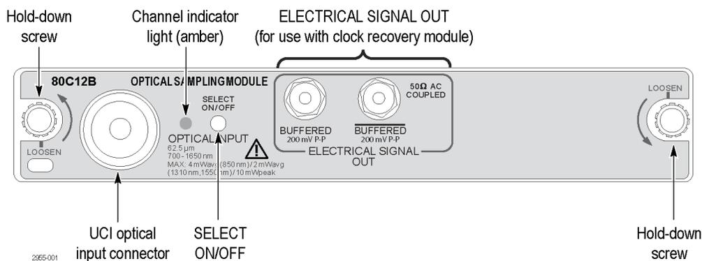
Figure 3: 80C12B optical module front panel
