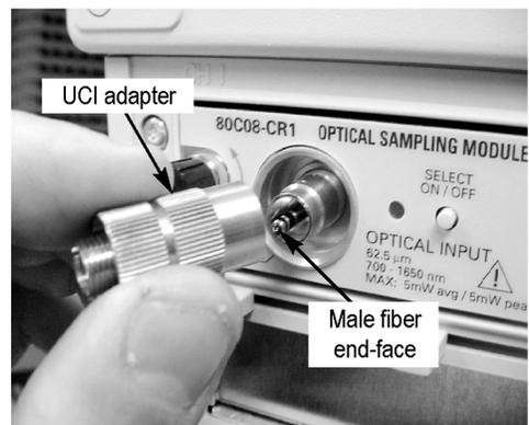
**Clean UCI adapter** 2. Clean contaminants from the inside wall of the hollow female-to-female ferrule alignment tube inside the UCI adapter.
