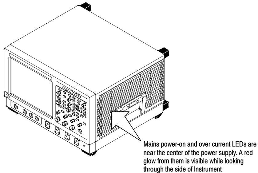
**Figure 6-36: Location of power-on and over current LEDs**
