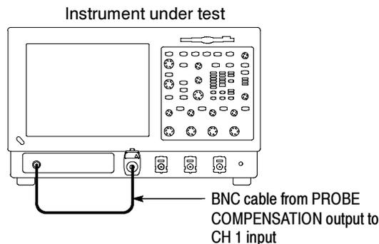
**Figure 4- 4: Setup for time base test**
