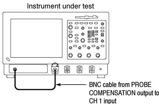
**Figure 4- 5: Setup for trigger test**
