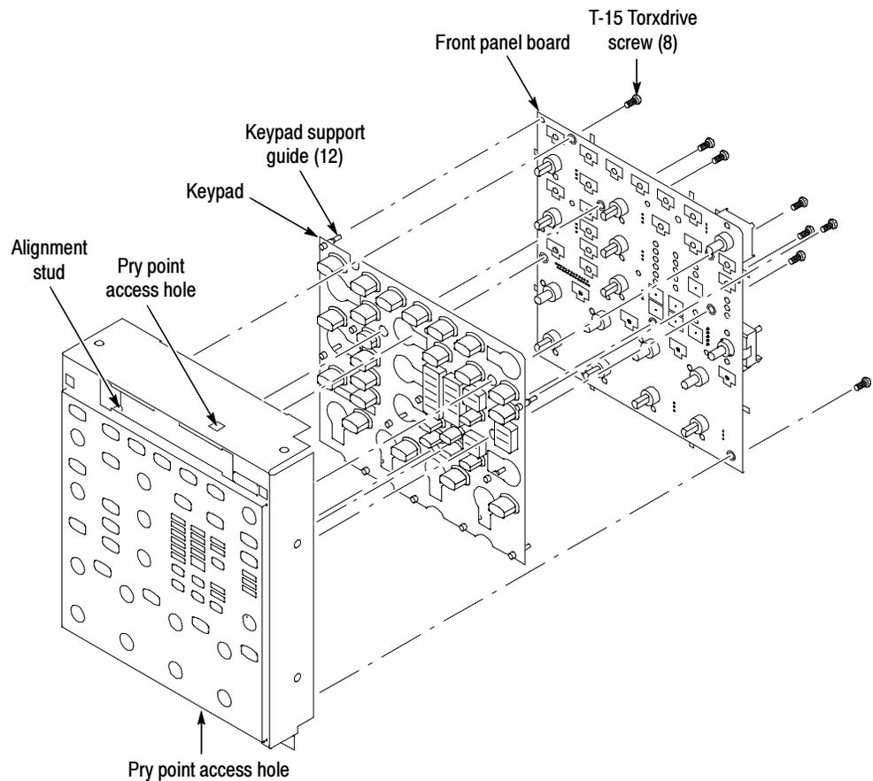
**Figure 6- 11: Front panel board and keyboard removal**
