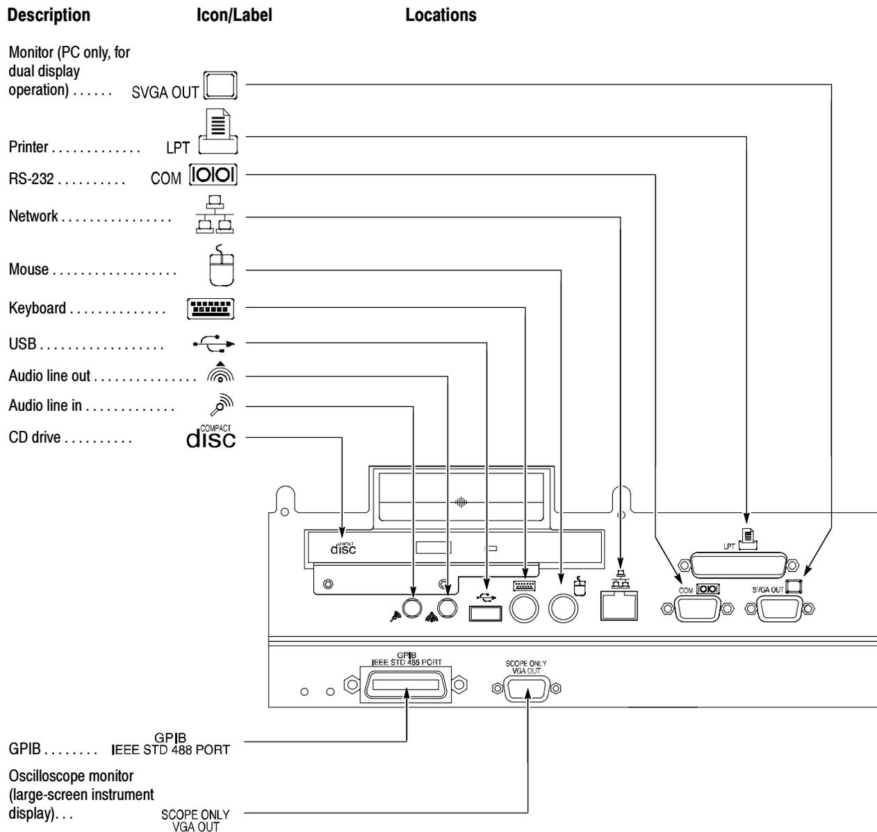
**Figure 2-1: Locations of peripheral connectors on rear panel**
