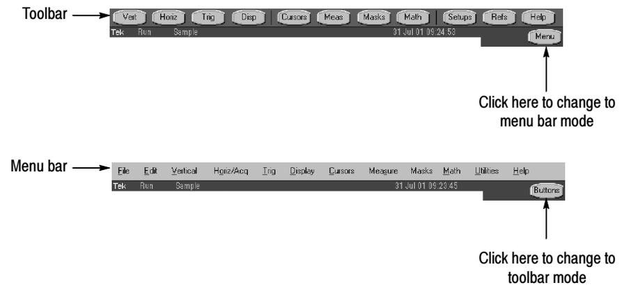
**Figure 4-1: Toolbar and menu bar (CSA7000 Series shown)**
