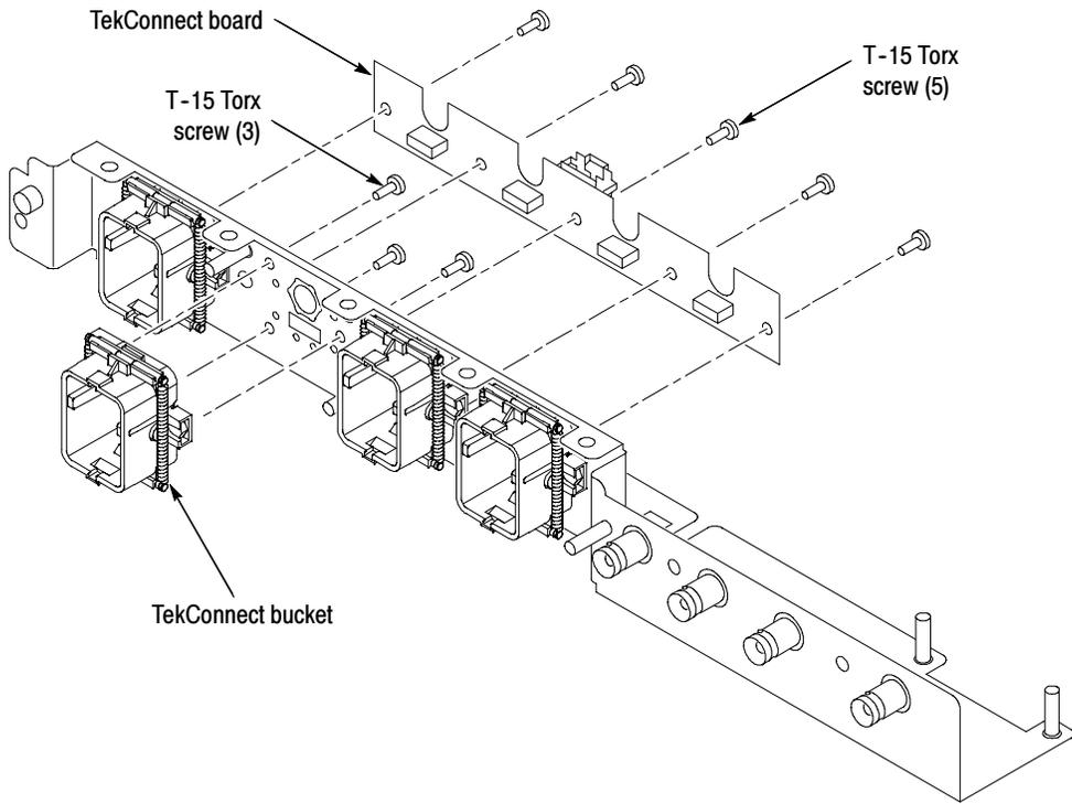
**Figure 6-34: TekConnect board and TekConnect bucket removal**
