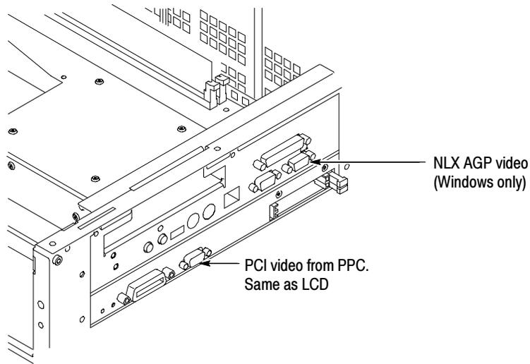
**Figure 6- 40: PCI and NLX video connectors**
