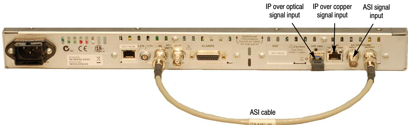
Figure 44: Connecting the ASI cable - GbE interface
