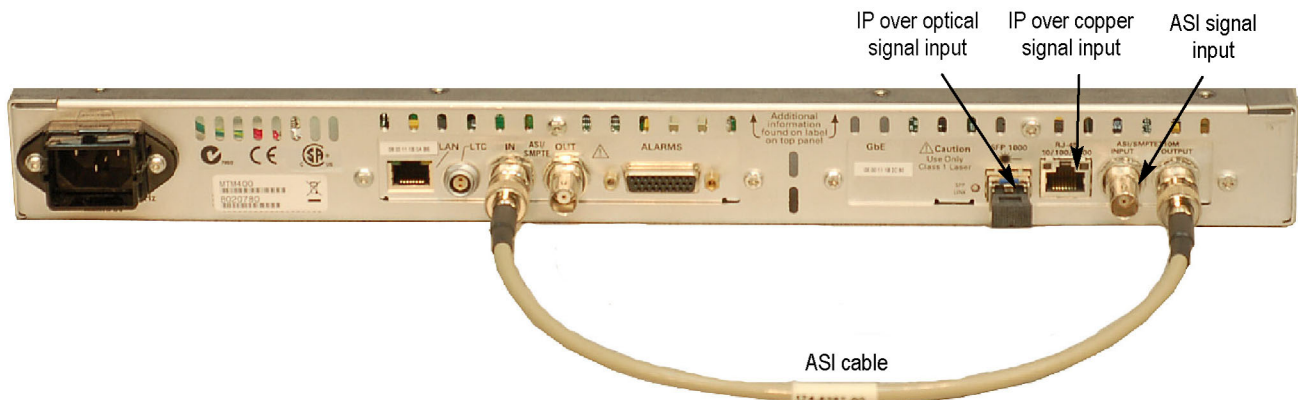
Figure 43: Connecting the ASI cable – GbE interfaces
