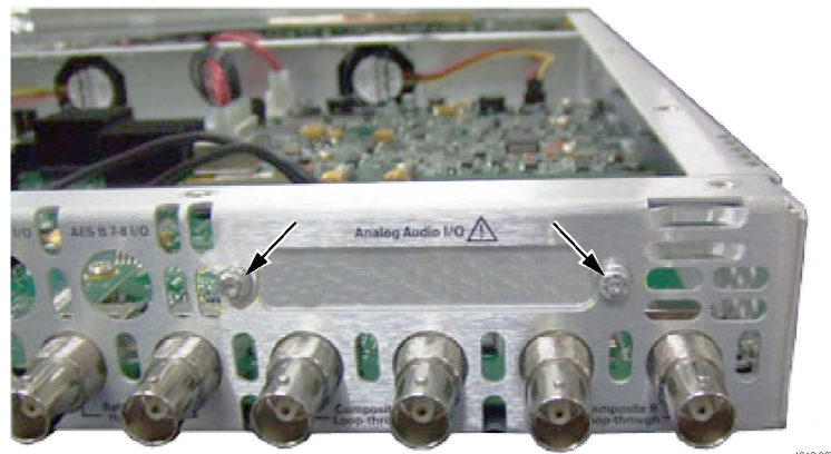
Figure 13: Remove blank cover for audio connector
