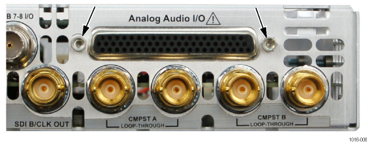
Figure 16: Audio connector retainer posts
