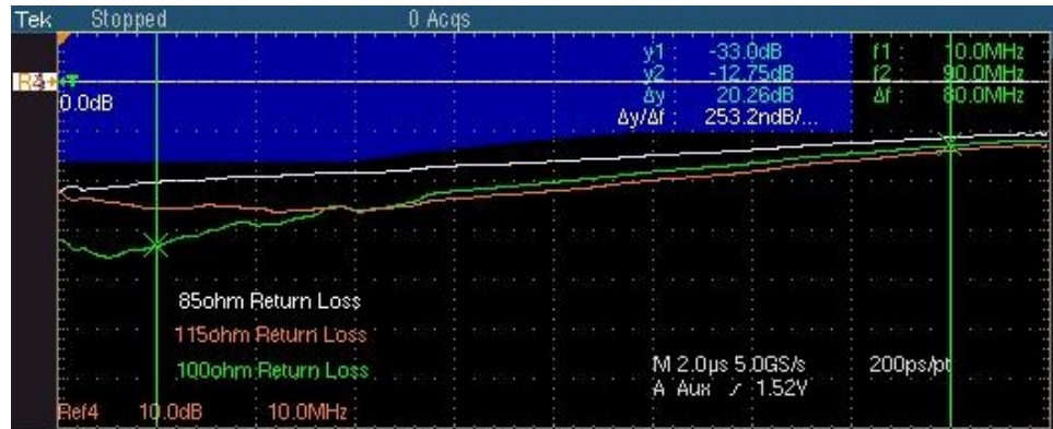
Figure 9-18: Waveform for 100BASE-TX Return Loss Transmitter
