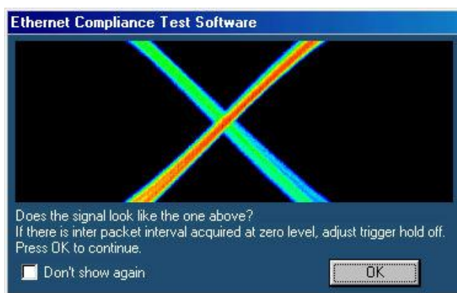
Figure 10-15: 10BASE-T Jitter with cable user control
