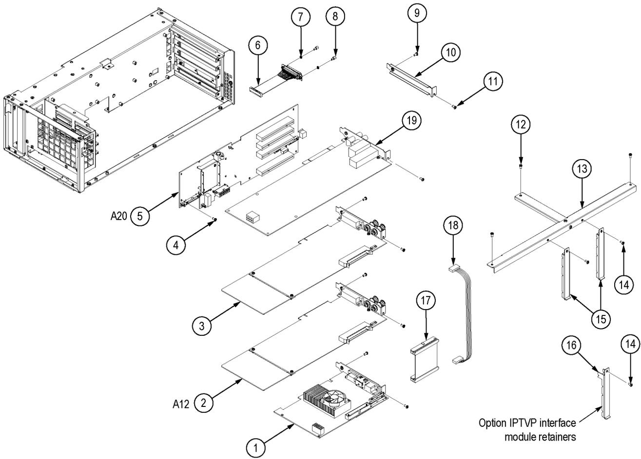
Figure 5-3: Internal modules
