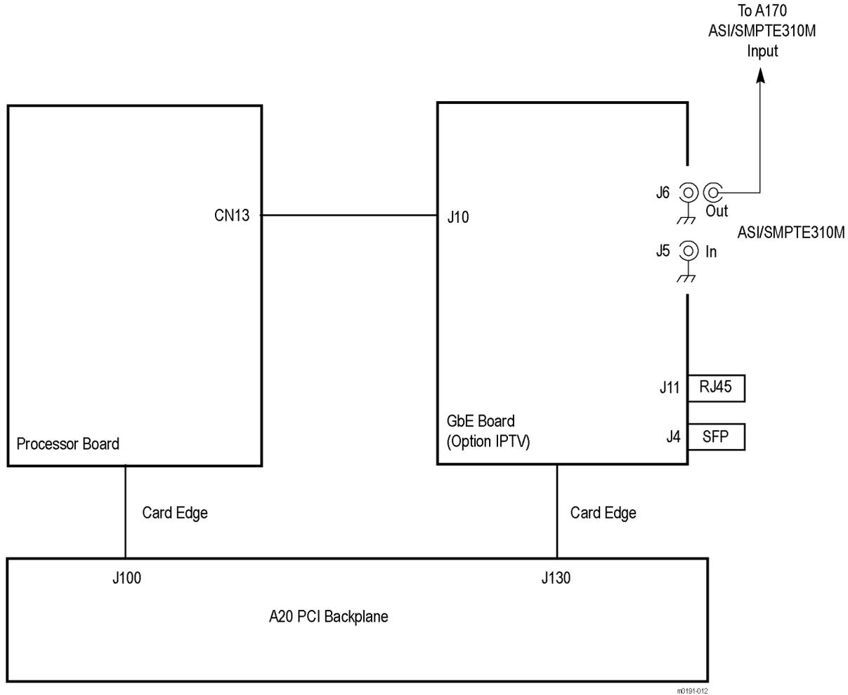
Figure 4-7: Option IPTVP (GbE) Interface module connections
