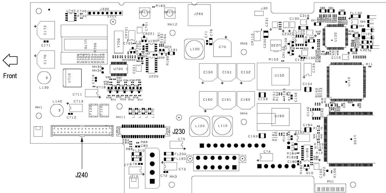
Figure 3-25: A20 PCI Backplane board view-right side
