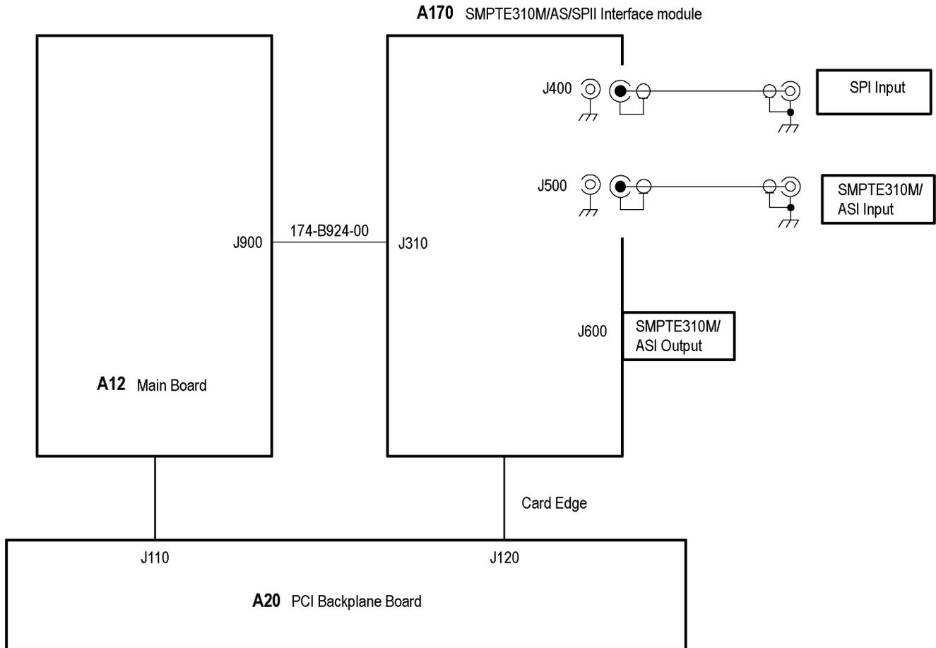
Figure 4-6: A170 SMPTE310M/ASI/SPI Interface module connections
