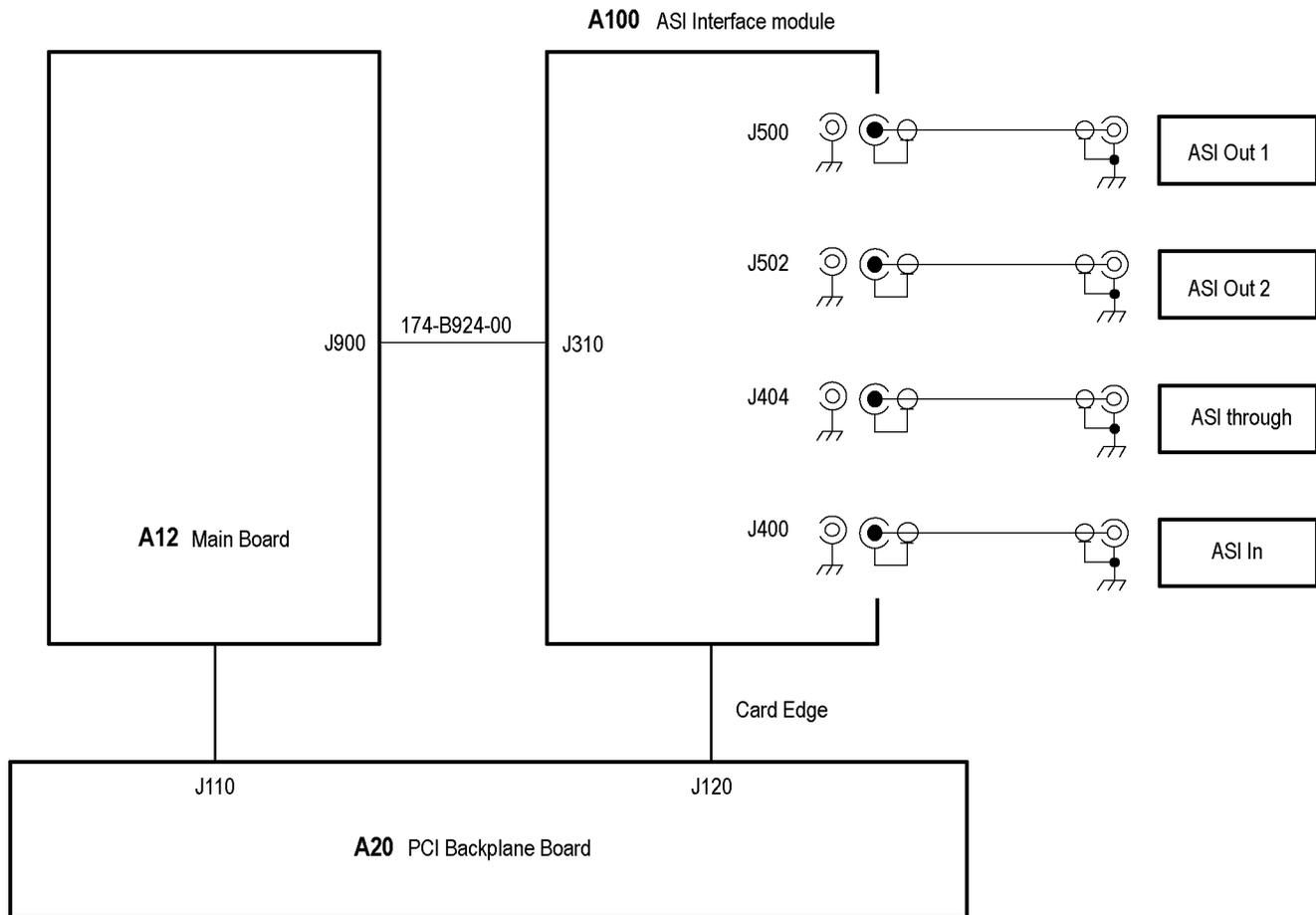
Figure 4-3: A100 ASI Interface module connections
