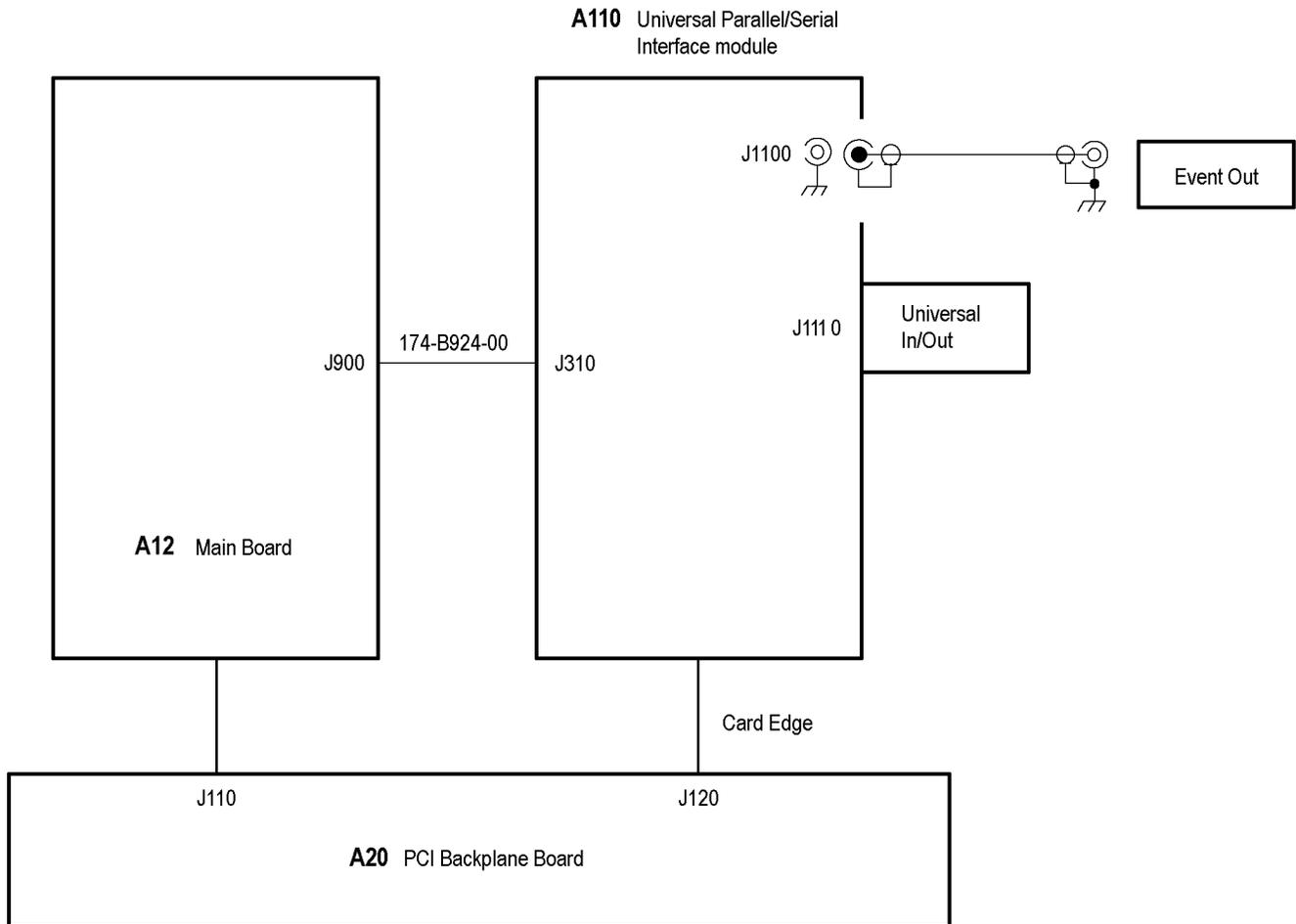
Figure 4-4: A110 Universal Parallel/Serial Interface module connections
