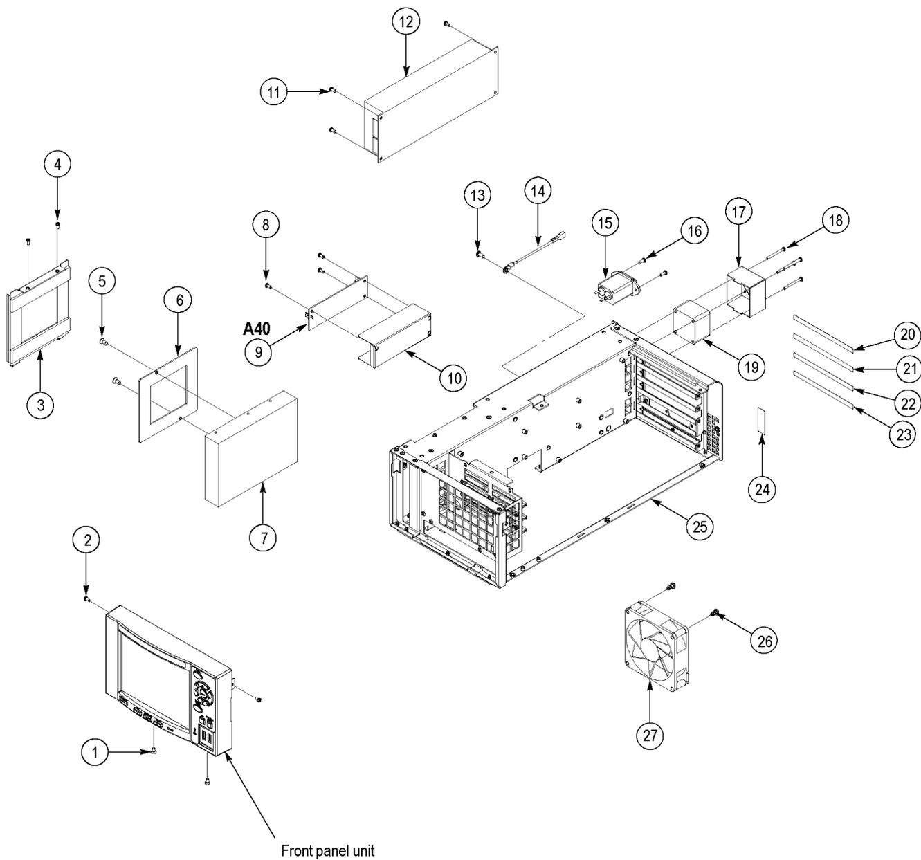
Figure 5-2: Internal modules
