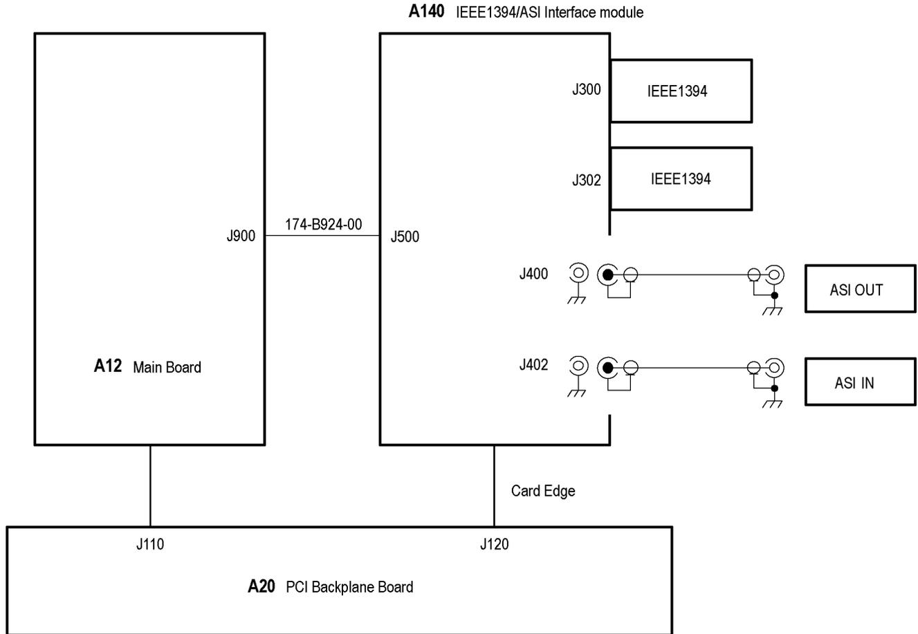
Figure 4-5: A140 IEEE1394/ASI Interface module connections
