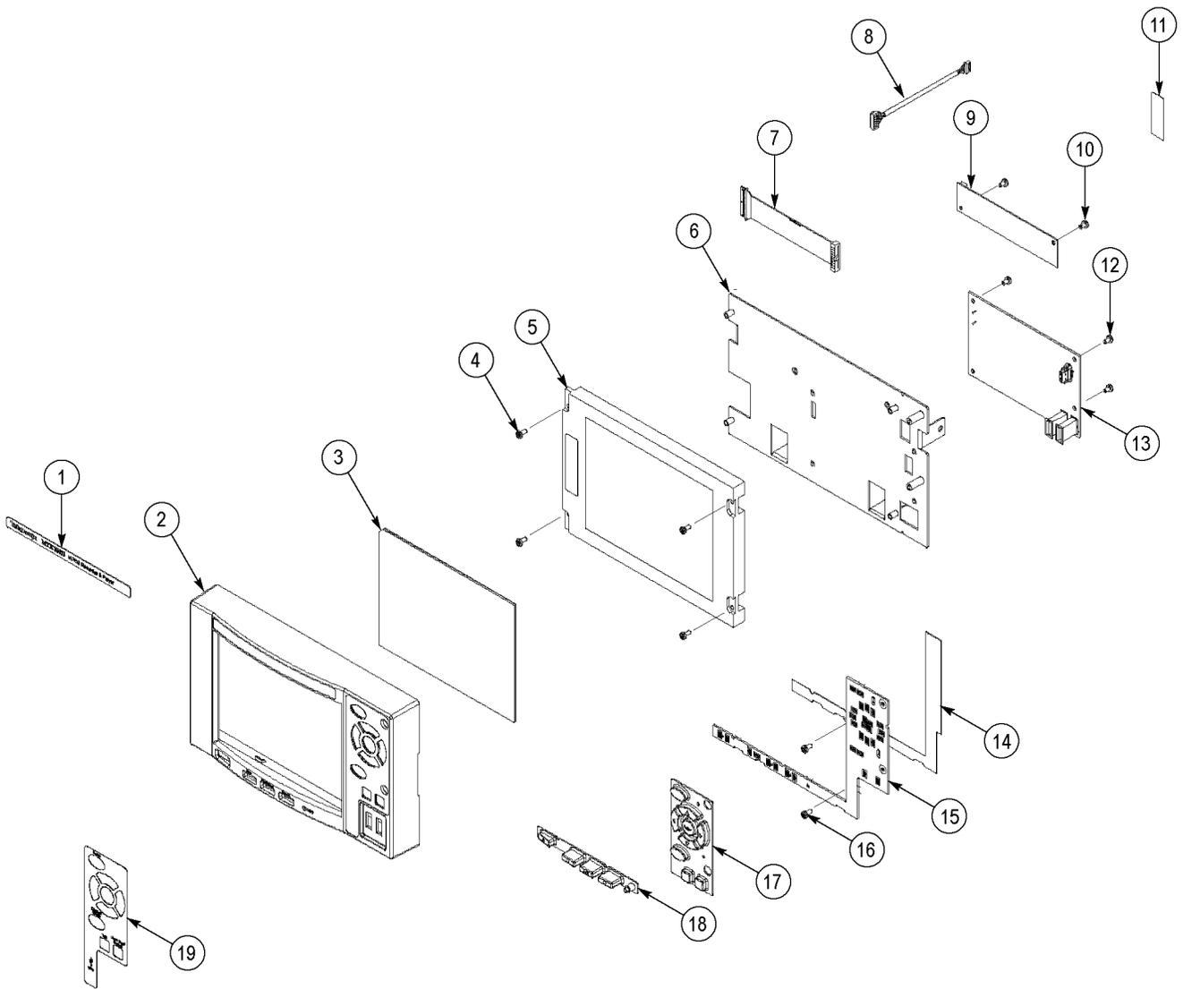
Figure 5-4: Front-panel unit
