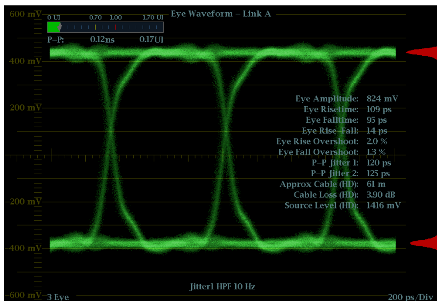
Figure 31: Eye display in single tile mode (full-screen) with histogram
