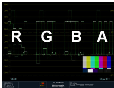
Figure 14: Dual Link information placement in waveform display
