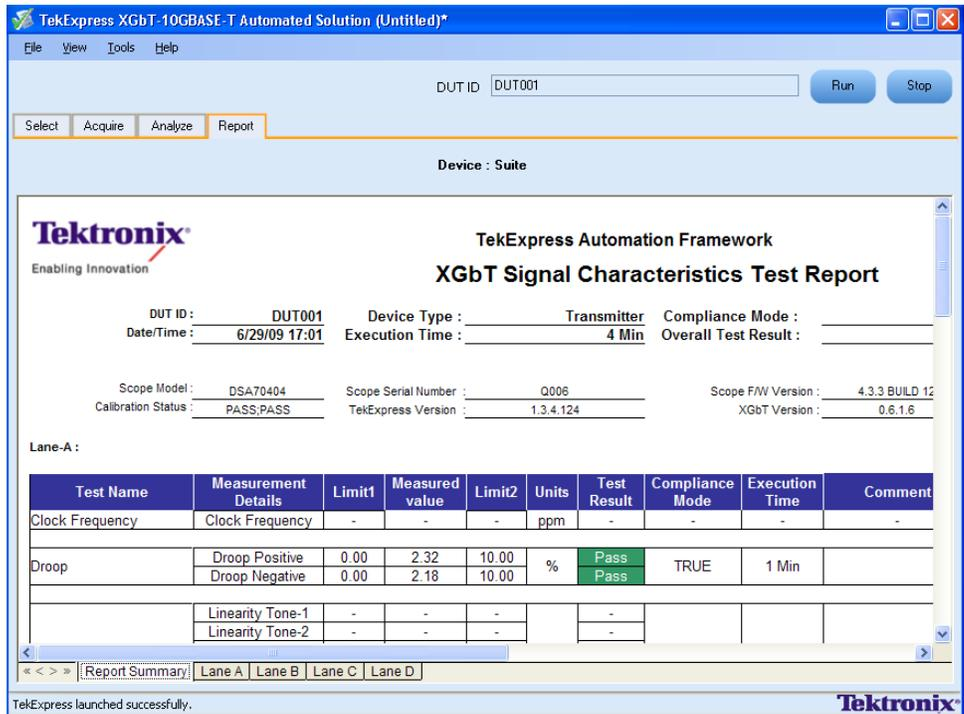
Figure 8: Report panel after Droop Measurement is Run
