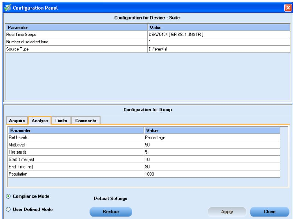
Figure 5: Configuration panel to set the Droop Parameters
