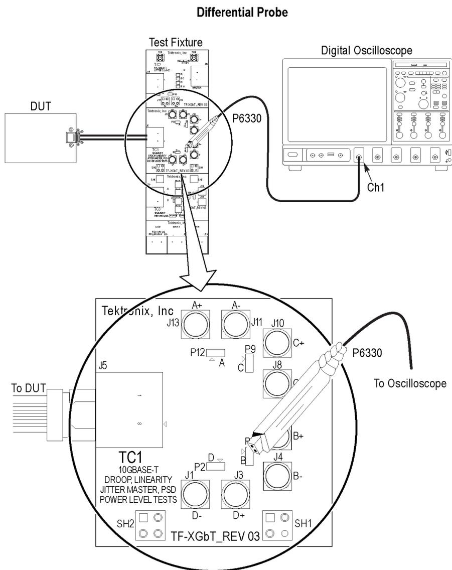
Note: When using high input impedance differential probe, ensure that each of the single ended lanes is terminated with 50 Ω.
