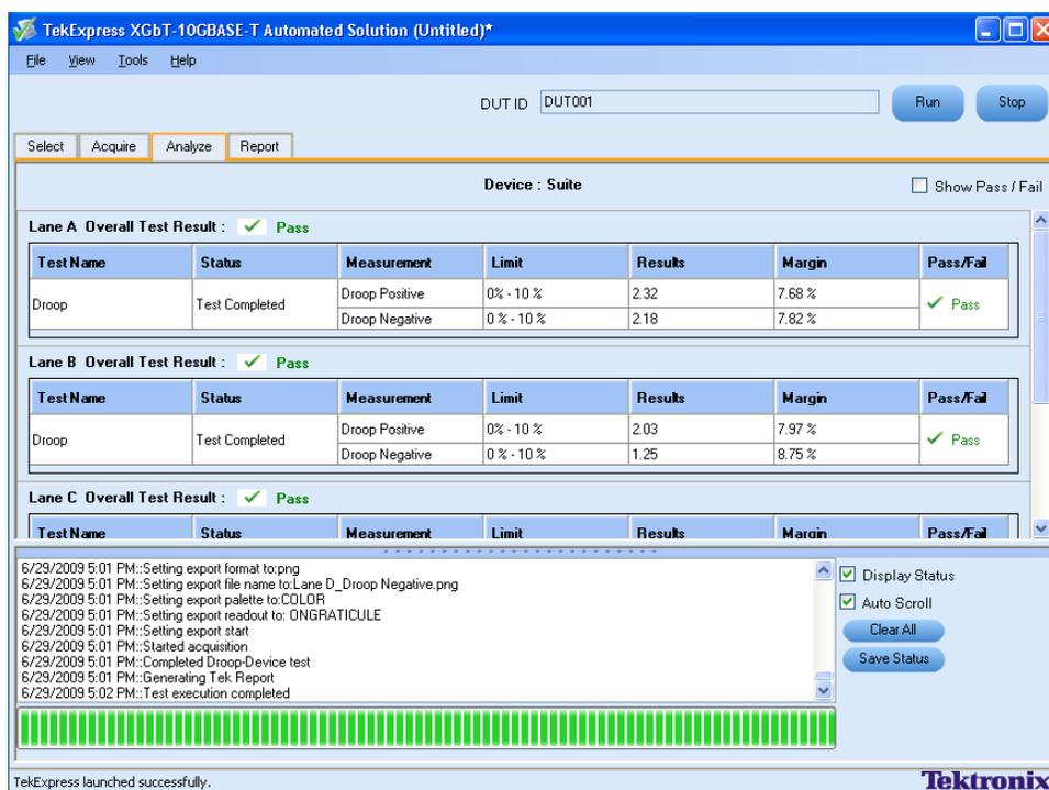
Figure 7: Analyze panel after Droop Measurement is Run
