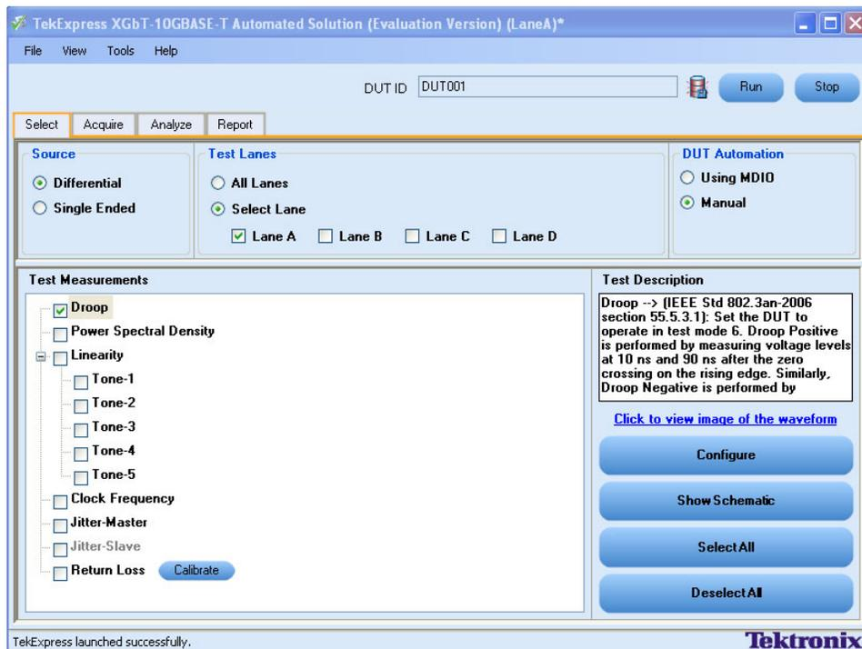
Figure 4: Select Panel with Droop Measurement Selected
