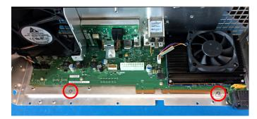
7. Lift the front half of the carrier interface assembly off the rear case enough to clear the mounting screw posts, and slide the carrier interface assembly out of the instrument. There is slight resistance from the spring clips on the rear panel
