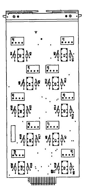
Figure 4-1. Model 7066, Component Location Drawing
