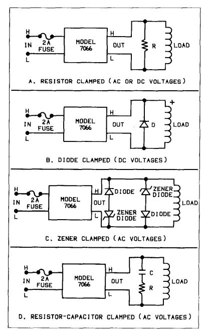
Figure 2-8. Limiting Inductive Reaction Voltage
