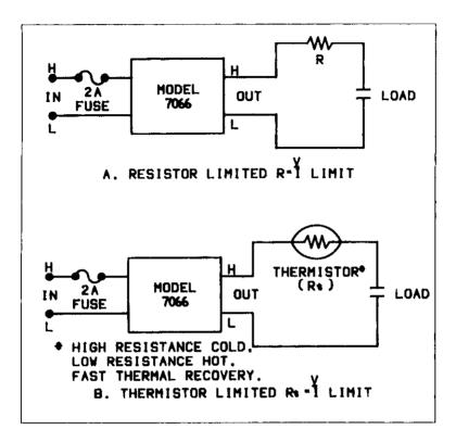
Figure 2-9. Limiting Capacitive Reaction Current
