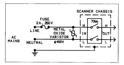
Figure 2-10. Clamping AC Mains Transients
