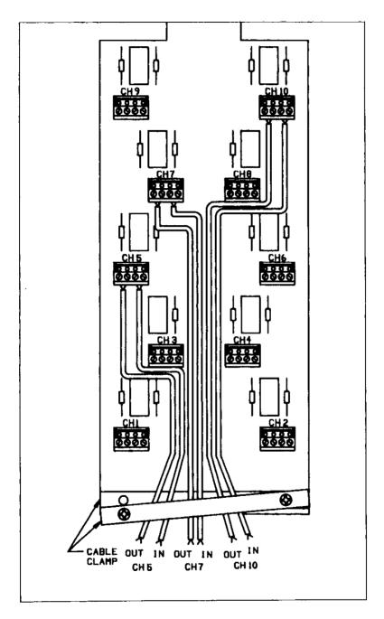
Figure 2-4. Typical Wire Routing
