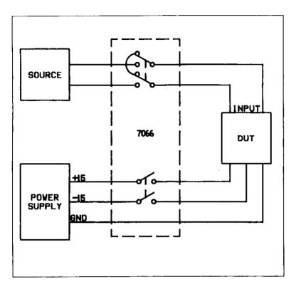
Figure 2-11. Switching Sources and Supplies
