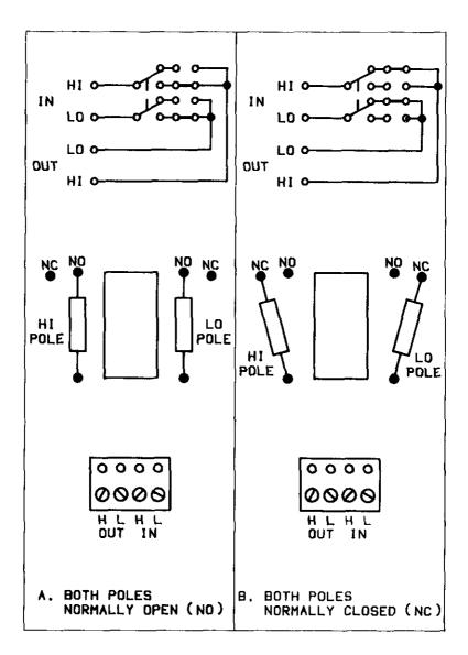
Figure 2-1. Jumper Positions for NO and NC Operation
