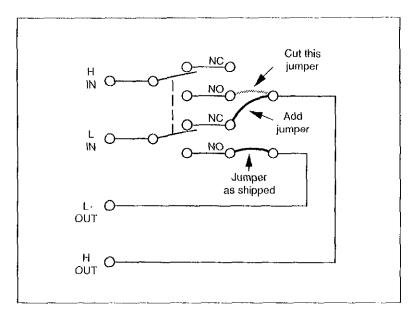
Figure 2-5. SPDT Configuration
