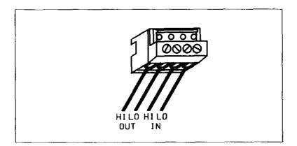
Figure 2-3. Quick Disconnect Terminal Block
