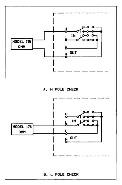
Figure 3-1. Performance Verification Setup
