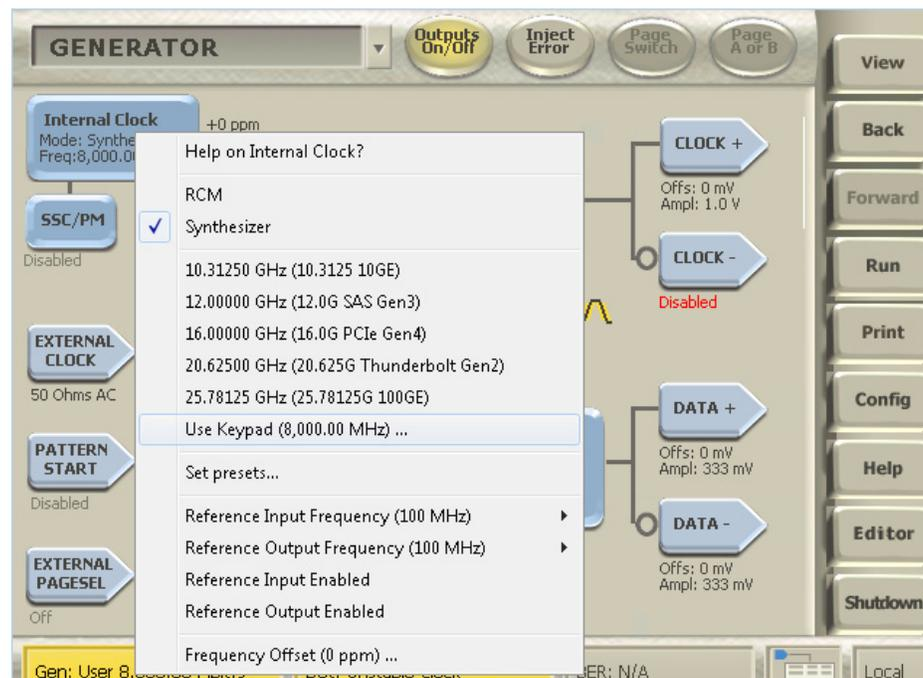
**NOTE.** By default the Internal Clock uses the Synthesizer mode where you can use one of the internal clock selections or select a value from the pop-up keypad. Refer to the online help for more information on the Internal Clock selections.
