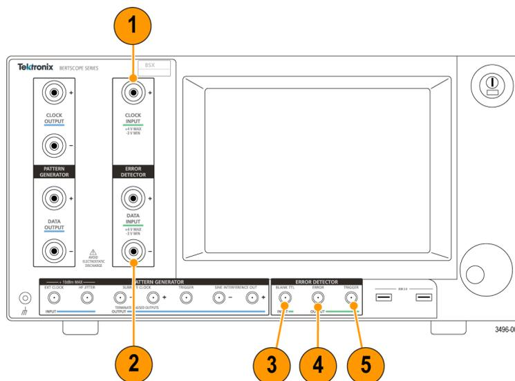
**Figure 4: Error Detector front panel connectors**
