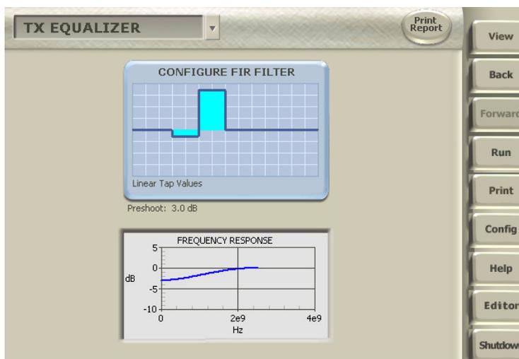
Figure 21: TX Equalizer view showing 3 dB preshoot
