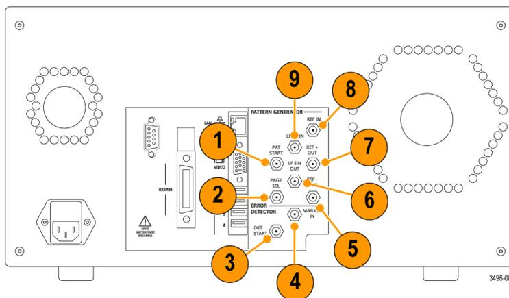
Figure 6: Rear panel BNC connectors
