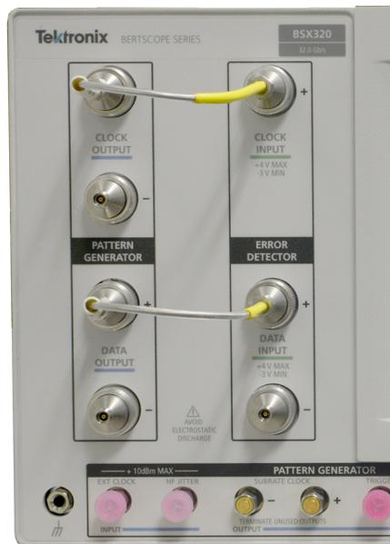
Figure 23: Front panel cable connections for the Pattern Sequencer examples
