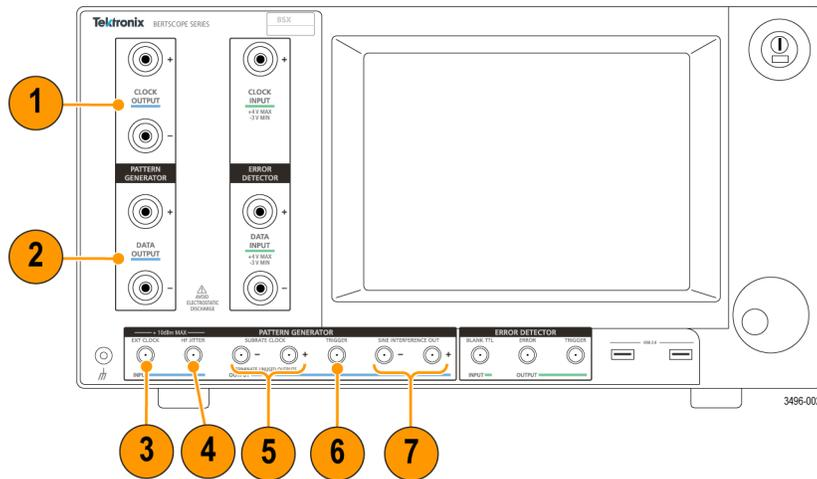
**Figure 3: Pattern Generator front panel connectors**
