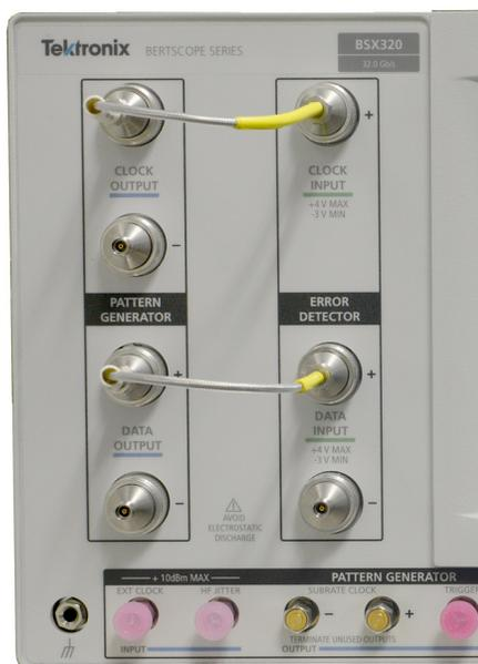
Figure 10: Initial front panel cable connections
