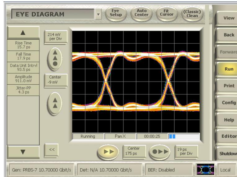
Figure 14: Typical eye diagram
