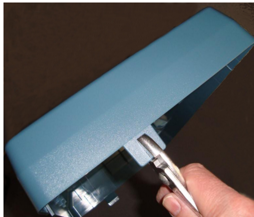
Figure 2: Removing tabs from the front protective cover
