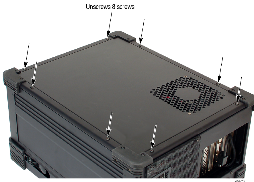
Figure 3: Remove rear panel
