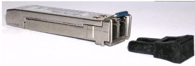
**Figure 7: Sample SFP optical module**
