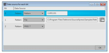
The selected modulation type determines the number of bits presented in the dialog screen. The selections available for each bit are the same available as described for the Single data source selection.
