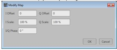
Adjust Offset, Scale, and Phase for I and Q.
