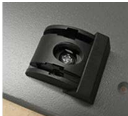
Figure 2: Remove feet from the instrument
