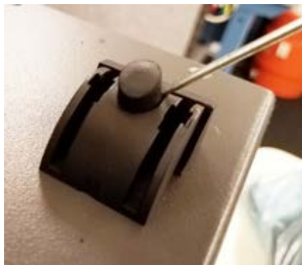
Figure 2: Remove feet from the instrument
