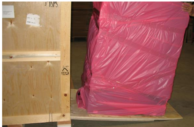
Figure 14: Sliding the system down the ramp
