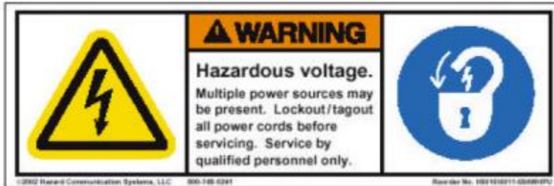
Figure 25: Hazardous warning label
