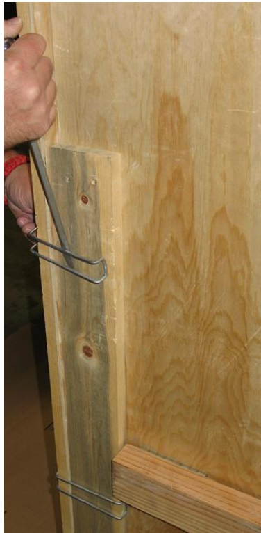
Figure 4: Removing the crate clamps
