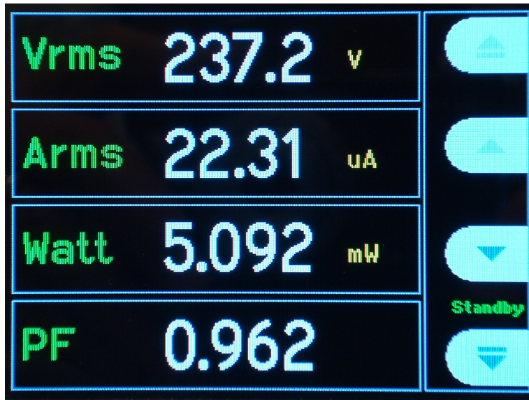
Figure 19: PA1000 measuring 5 mW in front-panel standby mode
