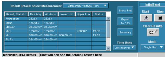
Figure 10 - Details View of Pk-Pk measurement.
