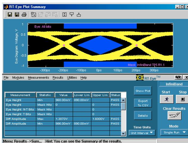
**Figure 9 - Result of the Differential Amplitude Measurement.**
