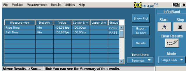
**Figure 12 - Results of Transition Time Test.**
