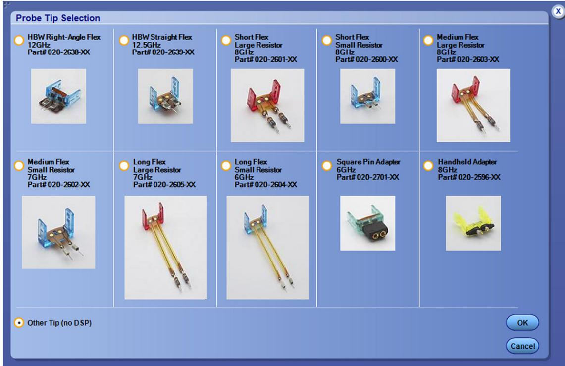
Shown below are the tips for P75xx family of probes. However, only the Performance Solder Tip is currently supported with S-parameter sets.
