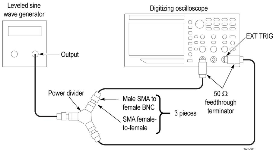
3. Set the oscilloscope **Vertical Scale** (volts/division) to **100 mV/div**.
