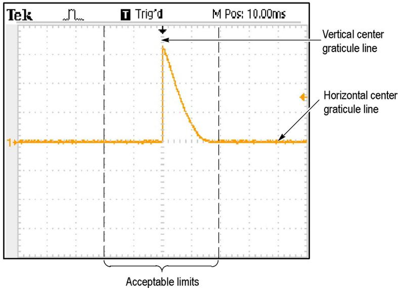
**NOTE.** One division of displacement from graticule center corresponds to a 25 ppm time base error.
