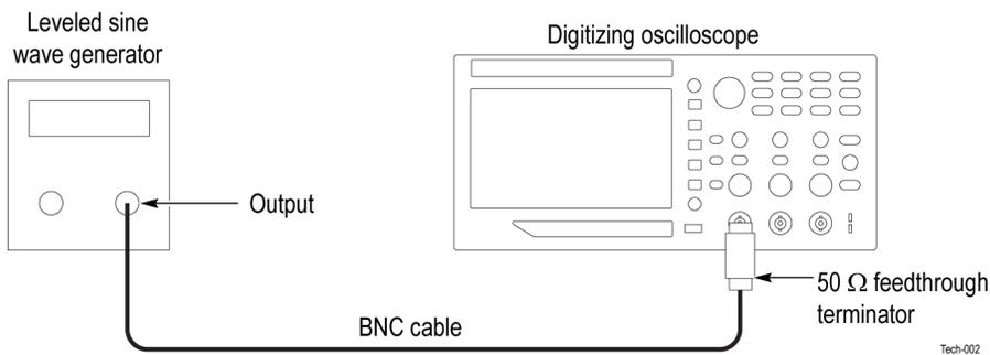
3. Set the oscilloscope **Vertical Scale** (volts/division) to **500 mV/div**.
