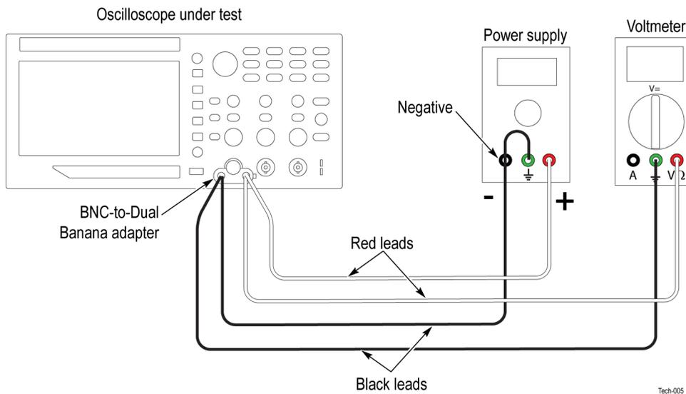
4. Set the power supply to the 1.8 V value shown in column A, the Approximate Test Voltage.
