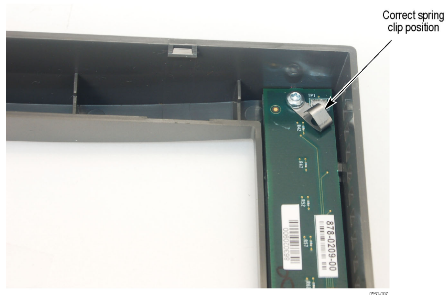
Figure 8: Correct spring clip position
