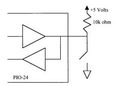
In Figure 2, the digital input is guaranteed to be pulled high because of the 10k ohm resistor. This implementation would work on both the old and new design of the PIO-24 and is the preferred implementation to avoid dependence on a specific level of input load current.
