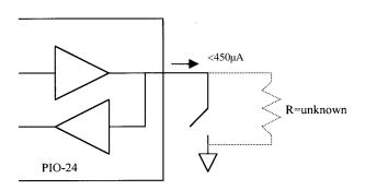
In Figure 1, the digital input would most likely float high with an older design board because of the higher input load current. When the switch is closed, the input will be pulled low. While this would work on an older design of the PIO-24, this is a poor implementation because the input load current can vary from one board to the next. In the case of a new design board, this would not work because of the lower load current.
