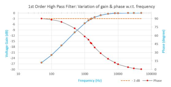
• Find out the cut-off frequency from the plot (where the gain drops to -3dB from its passband value)
