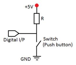
Arduino can read the input pin level (HIGH or LOW) and detect the switch press.
