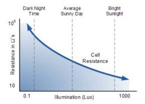
The light variation can be 'measured' by using LDR with another resistor as voltage divider circuit. ADC of Arduino can be used to measure the voltage change (due to variation in intensity of light on LDR).
