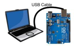
Launch Arduino IDE and ensure correct USB port number and Board name for establishing the connection
