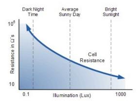
Change in resistance can be converted in to voltage variation by voltage divider implemented using LDR and a fixed resistor.
