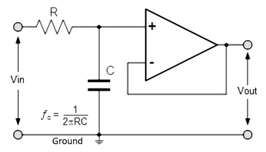
Choosing R = 1k Ohms and C = 0.1uF, cut-off frequency will be 1592 Hz
