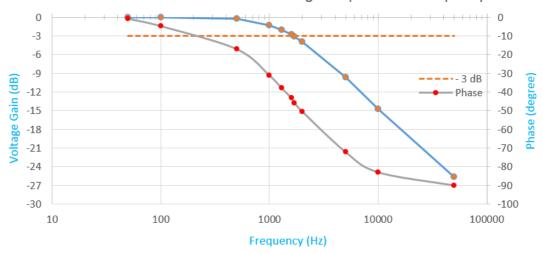
• Find out the cut-off frequency from the plot (where the gain drops to -3dB from its passband value)
