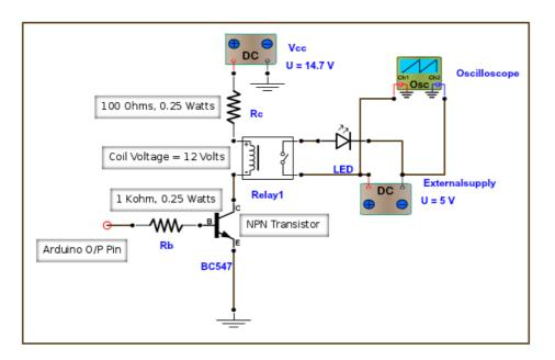
• Build the circuit connection as per the given circuit diagram.
