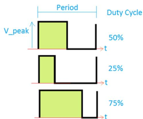
Area =  $V_{peak} * \text{duty cycle}$  Volt-sec
