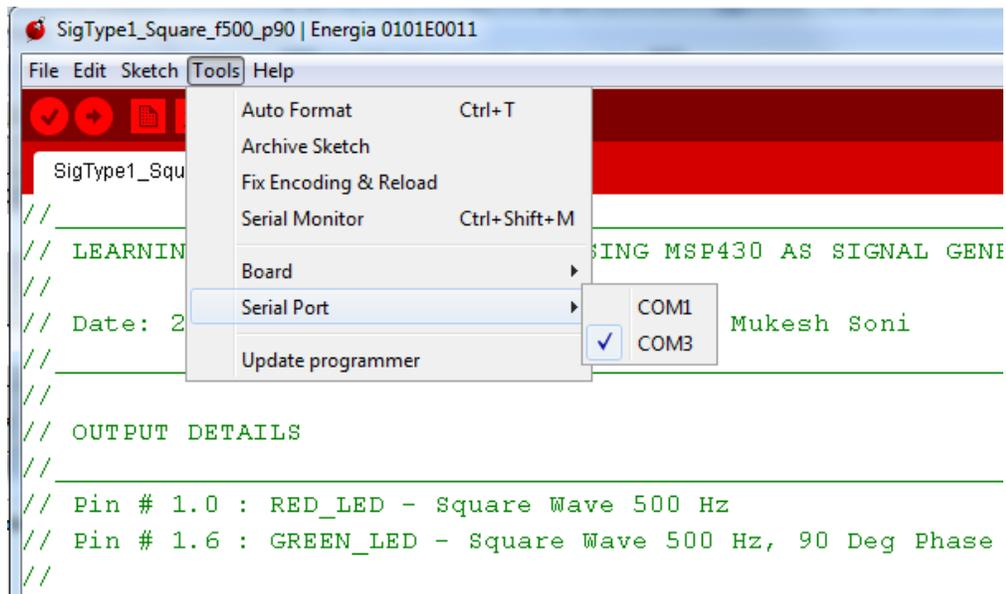
**STEP: 7.** Once the setting is complete, we are ready to download the program on MSP430 Launchpad board. We can test the setup by programming MSP430 Launchpad board with an example code (sketch). Go to : **File > Examples > 1.Basics > Blink**
