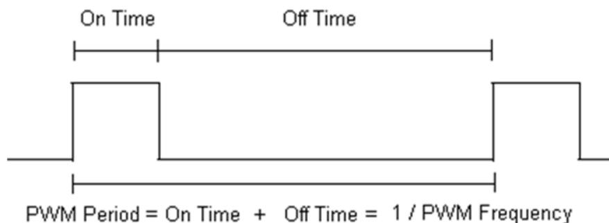
$$\text{Duty Cycle} = \frac{\text{On Time}}{\text{PWM Period}}$$
