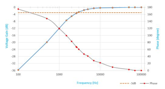
• Find out the cut-off frequency from the plot (where the gain drops to -3dB from its passband value)
